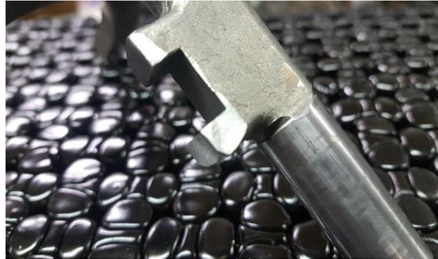
You will want either silicone or use the factory transfer case lever housing gaskets.
