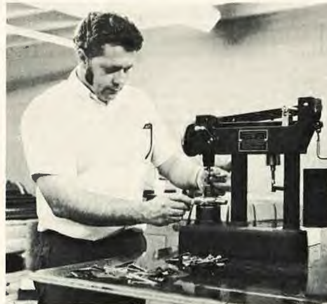
Chuck Buck sets up Rockwell test equipment for author to conduct hardness tests on steel used in broadheads. The unit measures hardness, comparing one type with another.
