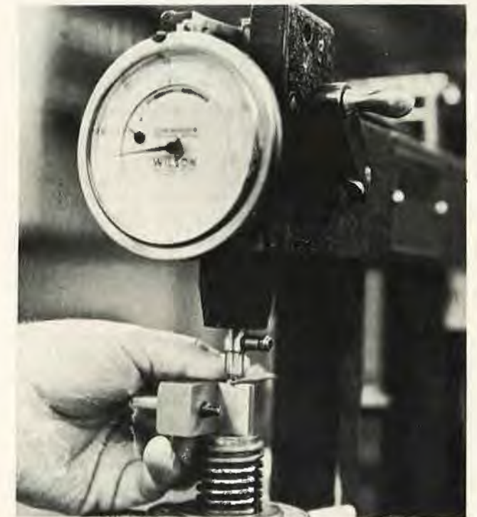
Broadhead is in position on the flat surface required for accurate reading. Lever on the left is lowered and the scale in front will read the hardness of the metal.
