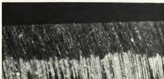
Another broadhead sharpening device is the Razor Edge, consisting of clamp that holds two-bladed head, set of two stones. Allen wrench is used to tighten the head. (Below) This is edge of a Bear Razorhead after honing on the Razor Edge unit. Note the sharp bevel, cutting edge.
