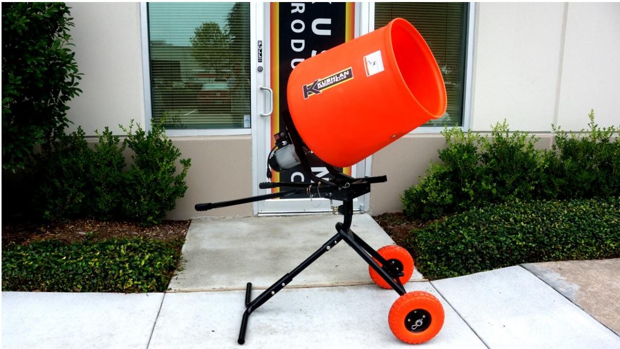
**Step 19** - Rotate to 180° to the lock out position. To dump, raise the handles and dump the concrete out onto either a wheelbarrow or directly onto the work you are doing. By pulling the swivel latch and rotating at 180° to the lock out position, the mixer will rotate 360°.
