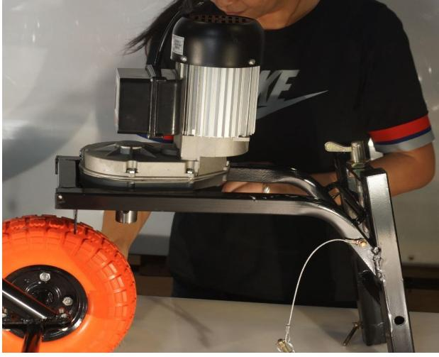
**Step 9**— Install gear motor on the tilting main frame.
