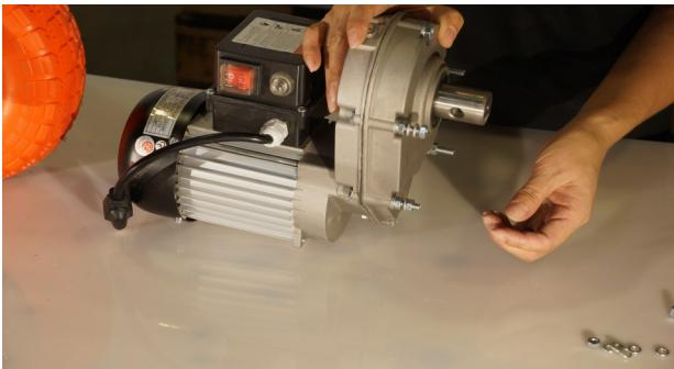
**Step 5**—Take off outer nuts, flat washer and spring washer.
