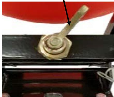
**Step 18** - The mixer can be wheeled with a full load of concrete in the upright position however it's designed for a smooth flat surface. To do so, note both the dump latch and swivel latch must be engaged to wheel concrete in the upright position.
