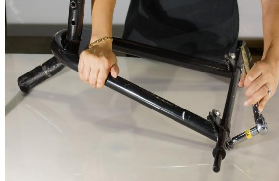
**Step 2—**Bolt axle to the main lower main frame.
