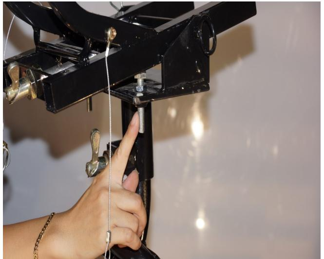
**Step 12** -Adjust the nuts and bolts under the swivel support so the dump latch will operate smoothly.
