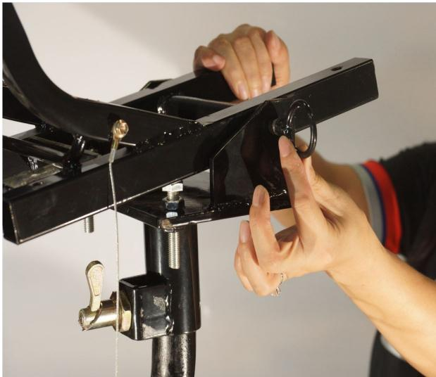
**Step 11**— Attached the tilting main frame to the swivel bracket by inserting the pivot pin and securing with an R clip.
