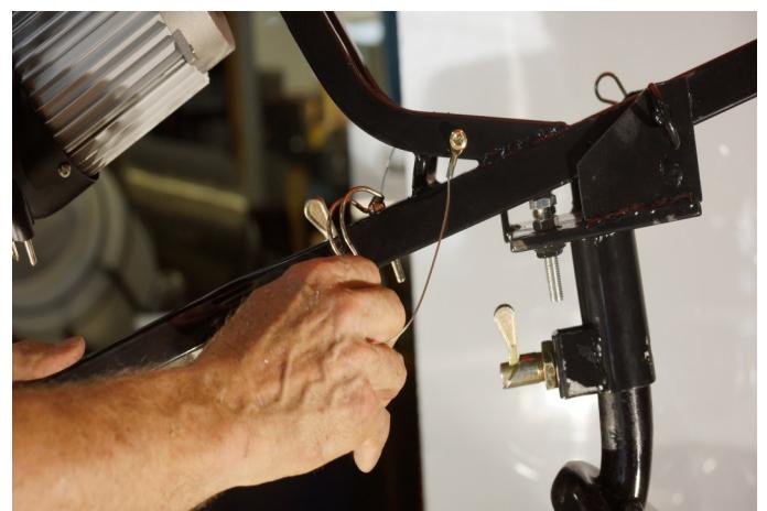
**Step 16**— Install the large bolt and tighten the Lock nut.
