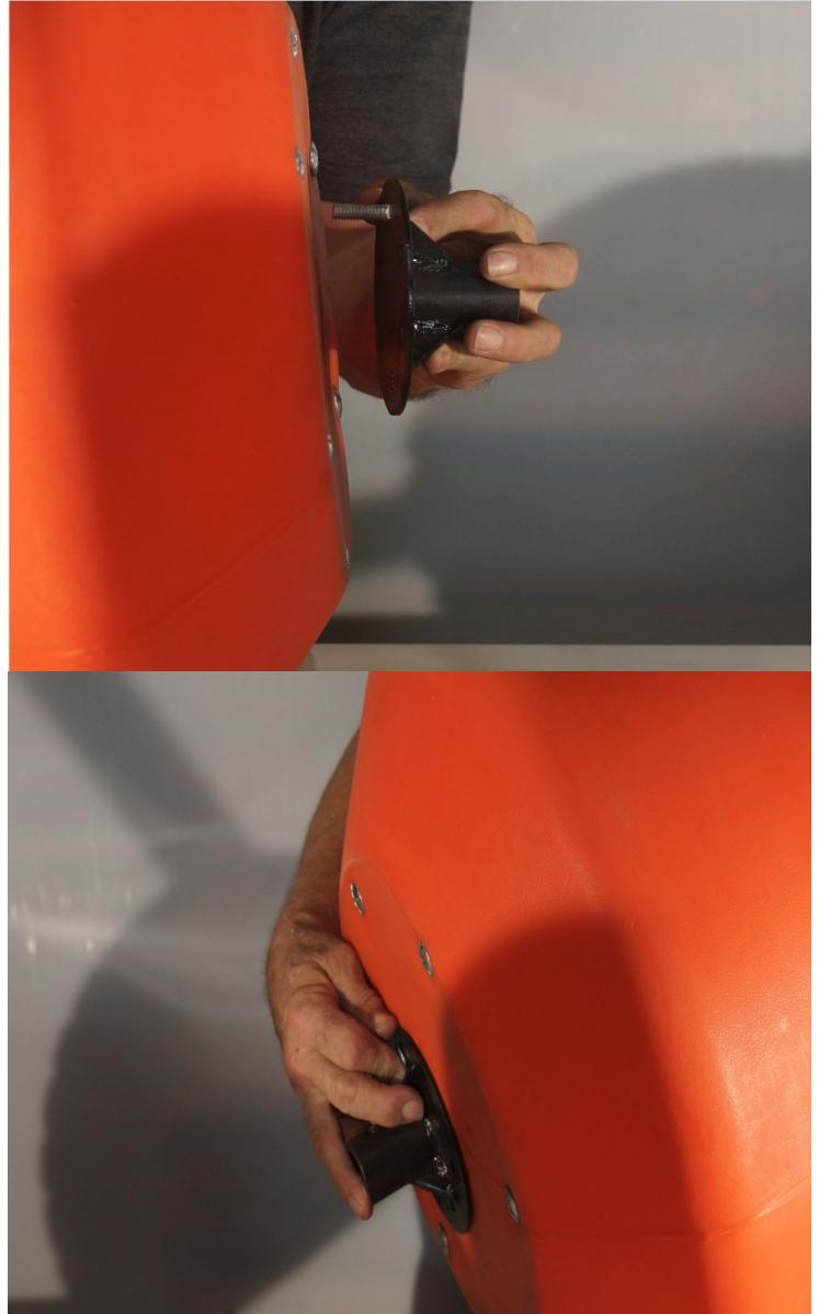
**Step 14**—Install the bushing to the back of drum then install the nuts on the inside of the drum. Tighten the inside nuts to secure the bushing.
