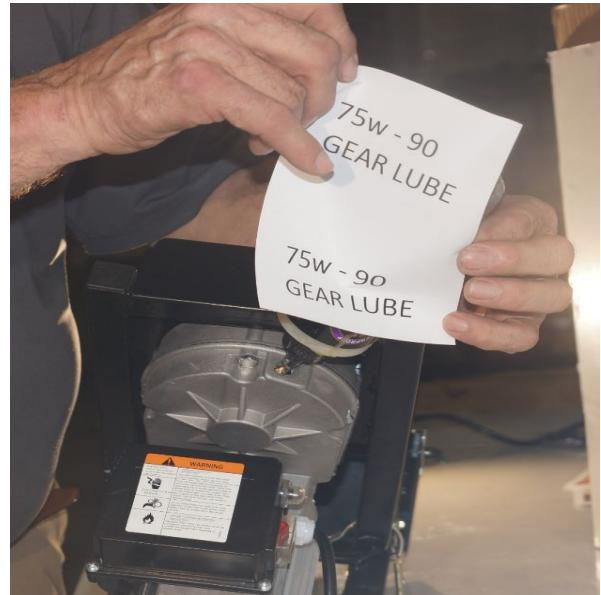
**Step 8**— When changing oil, use a squeeze bottle, measure 4 ounces of 75w-90 SAE gear lube and squeeze into plug hole.
