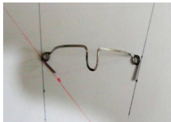
Additional line is drawn with a red pen to determine the amount of activation
