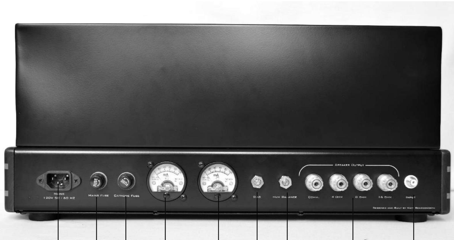
4. Mains Input      5. Mains Fuse      6. Cathode Fuse      7. Bias Current Meters      8. Bias      9. Hum Balance      10. Speaker Outputs      11. Input
