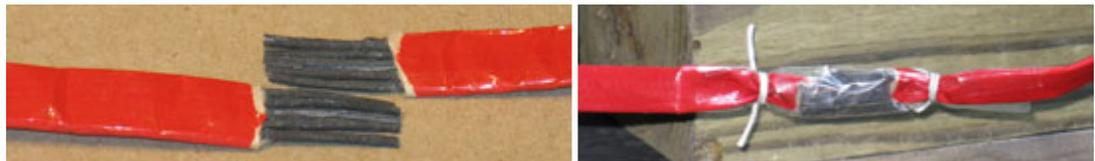
**Positive Disconnect Section Constructed in Quickmatch Leader**
