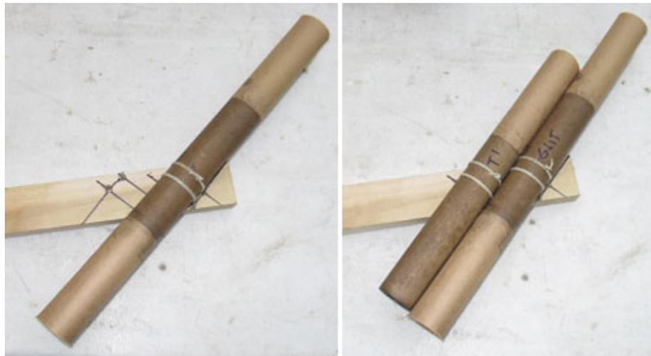
A quickmatch passfire is tied into the passfire end of the glitter driver and over into the thrust end of the Ti one.
