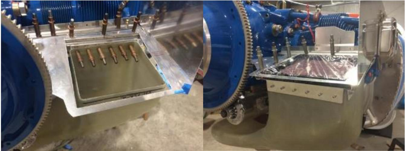
Air Intake for the New Demonstrator Lightning XS
