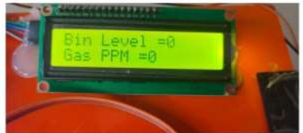
Fig. 10. LCD display bin and gas level
