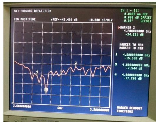
Fig 13: The input reflection coefficient S11
