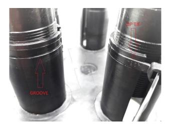
5. Reinstall the complete assembly again and the installation is complete. You need to remove the zip ties only if you want to reinstall the caps to a different style rims.
