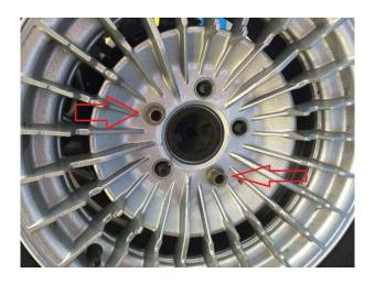
2. Install the plastic lower bracket, taking care to install it in such a way that the larger holes correspond with the original nuts previously installed, so that they can pass through. Then fix the bracket to the wheel with flanged bolts supplied in correspondency of the three bigger holes
