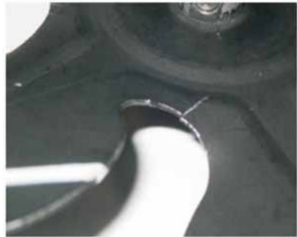
Figure 6. Laboratory Test Blade after cracking.
