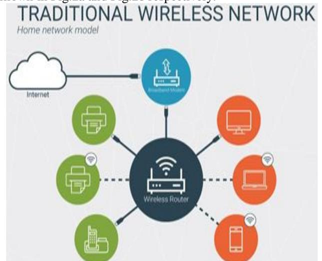
Figure 2(a): Traditional Wireless Network Diagram [2].
