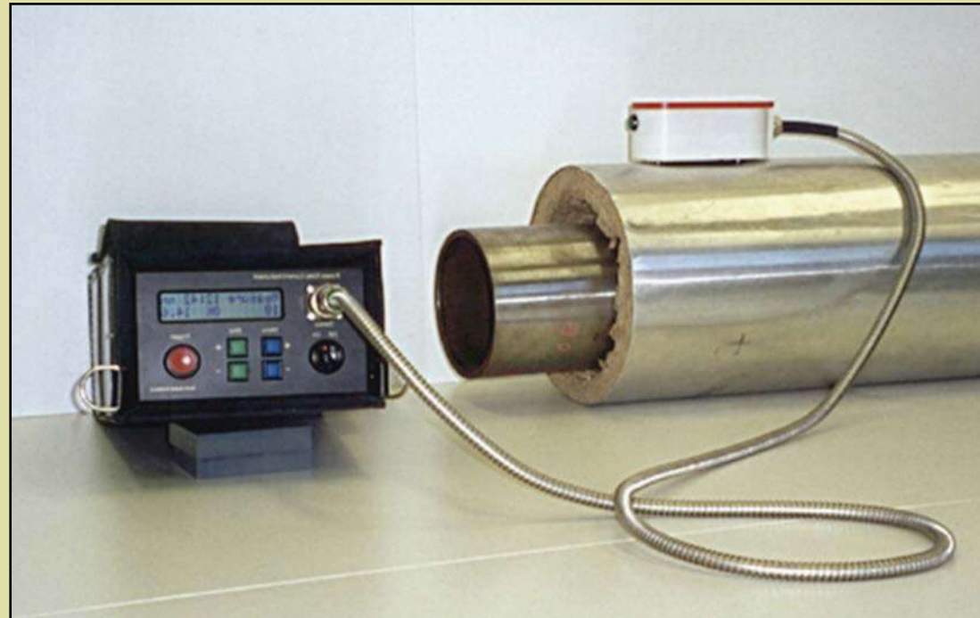
PEC instrument developed by Shell
