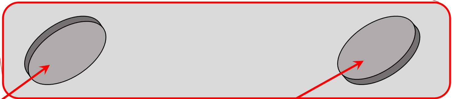
Raised Ejector Pin Mark
