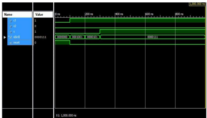
Fig.10: Simulation results of proposed 7:3 counter using reversible logic gates.
