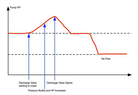
With a PD pump, a blocked outlet will increase pressure in the pump and the HP will increase. The diagram above shows a discharge valve starting to close and the HP starting to increase with pressure in the pump. When the valve again opens, the HP drops back down to the normal pumping power. When Flow is lost, the pump motor goes unloaded. The HP will drop to almost an idle condition on the pump motor until the pump heats and trouble occurs.
