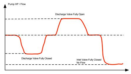
Pump Motor HP will change with Flow. As shown above, as flow is restricted using the discharge valve the HP will change proportionally. With the discharge valve fully closed, DEAD HEADED, some fluid remains in the pump and the power will not drop as low as compared to when the inlet valve is fully closed. With the inlet valve fully closed, NO FLOW, the pump will be empty and the power will be almost an idle condition on the pump motor before the pump starts to heat and trouble occurs.
