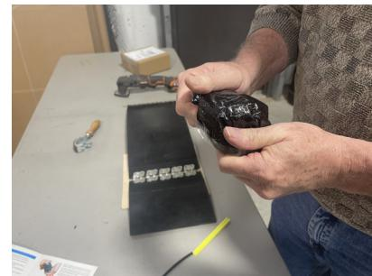
Mix by kneading and squashing the resin pack together until it starts to warm up (2-3 min).
