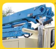
The 28Z-Meter boom features a simple mechanical rack and pinion design for improved weight distribution and easy maintenance. Putting the pump closer to the cab, rack and pinion slewing offers greater reach than rotation bearings on lighter weight models. Specially designed teeth in the system offer smooth rotation and prevent backlash in the swing gears.
