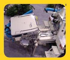
Fully removable, Putzmeister's modular bolt-on flatpack and hydraulic system combine versatility and servicing convenience. Pump cells can be switched out as jobs require or when maintenance is necessary. This feature also provides easier access to the S-Valve and shift cylinders.
