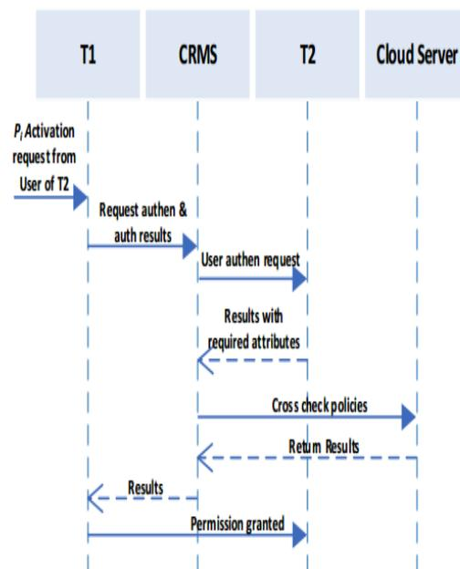
Fig.1: Sequence diagram for permission request in the cloud
