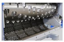
All Virtus shredders are equipped with a large diameter flat rotor. The knives are fixed in special knife holders fitted in machined pockets. Optional weld on hard facing is available for abrasive applications.
