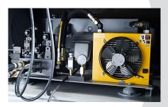
The X Series shredders feature a high powered twin speed hydraulic system. This system ensures maximum pressure when feeding material into the rotor and high speeds on the backstroke.
