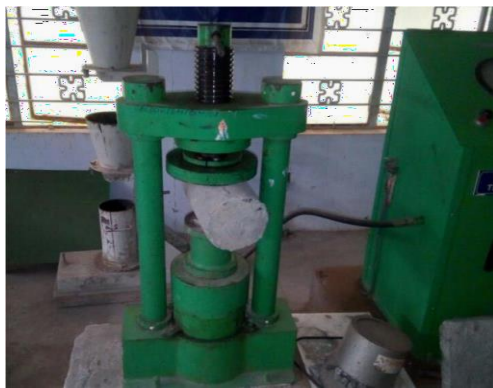
Figure 3: Split Tensile Strength Testing Machine
