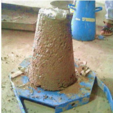
Figure 1: Slump Cone Test
