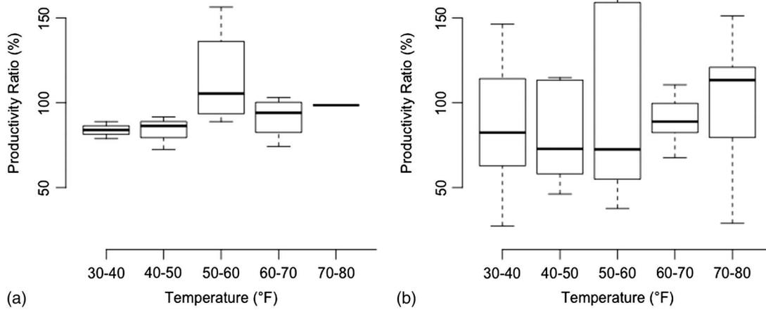
**Fig. 5.** Productivity of (a) masonry versus (b) other work (data from Thomas and Yiakoumis 1987)
