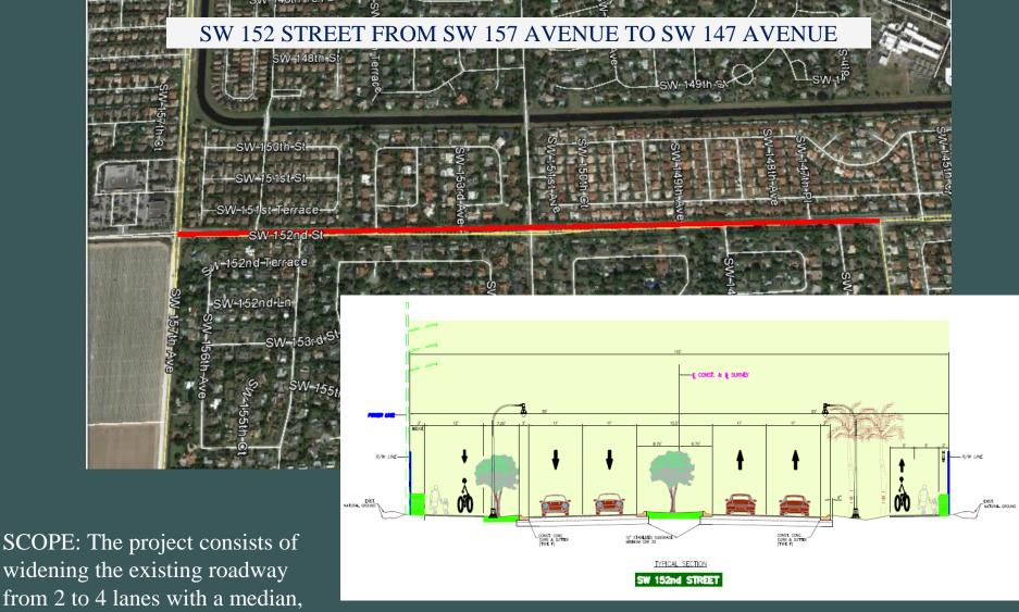
Shared use paths, curb and gutter, continuous storm drainage system, landscaping, signalization, pavement markings and signage, and decorative lighting.
