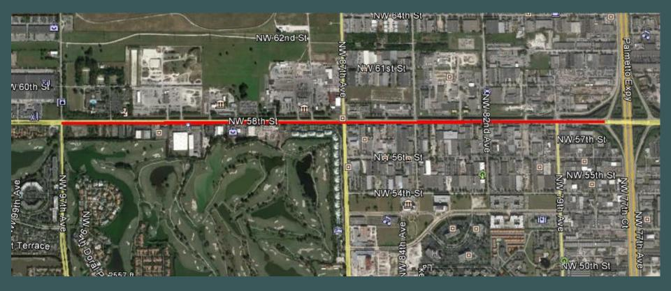
SCOPE: The project consists of master planning, public involvement, and preparation of complete construction plans to reconstruct the existing road to a 4-lanes roadway with continuous center turning lane, bike lanes, sidewalks, curb & gutters, storm water drainage system, pavement markings and signage, upgraded traffic signalization and roadway lighting.
