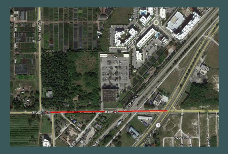
SCOPE: The project consists of widening the exiting roadway to a 2 lane divided roadway with center turn lane, bike lanes, on street parking, sidewalks, curb an gutter, storm drainage system, signalization, pavement markings, signage, and lighting.
