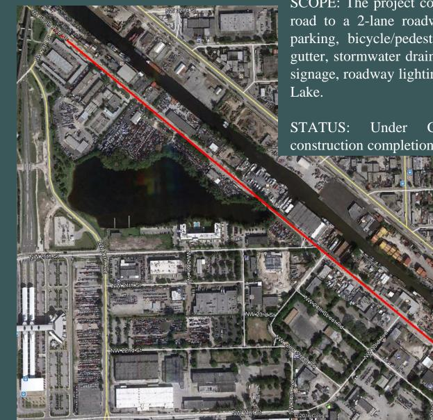
SCOPE: The project consists of reconstructing the existing road to a 2-lane roadway with center turn lane, parallel parking, bicycle/pedestrian shared use facility, curb and gutter, stormwater drainage system, pavement marking and signage, roadway lighting and bridge replacement at Palmer
