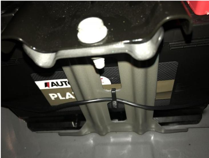
***Rear View of Battery and Recommended Strain Relief for Ground Wire***
