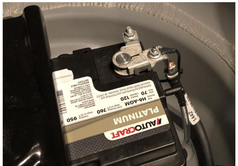
***Ground Wire Ring Terminal and Strain Relief***
