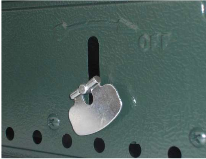
Figure 7 Auxiliary Burner Control
