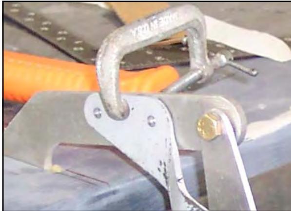
18. Install the aileron hinge to the flap bracket using AN3-6A bolts. Secure with AN365-1032 nyloc nuts and enough washer to allow the nut to tighten and show 1.5-3 threads of the bolt thru the nut.
