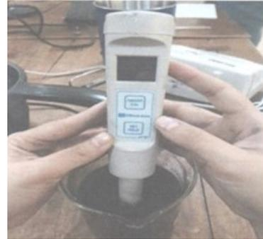
**Figure 6: Set-up measuring the pH nanofluid**
