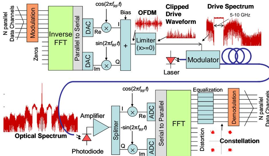
Fig. 3. Optical OFDM system block diagram including waveforms and spectra.
