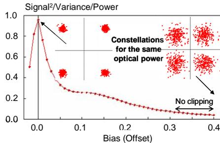
Fig. 4. Signal quality over optical power versus bias level.
