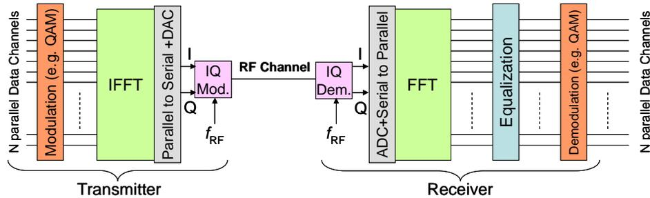
Fig. 2. Implementation of electrical OFDM using discrete Fourier transforms.
