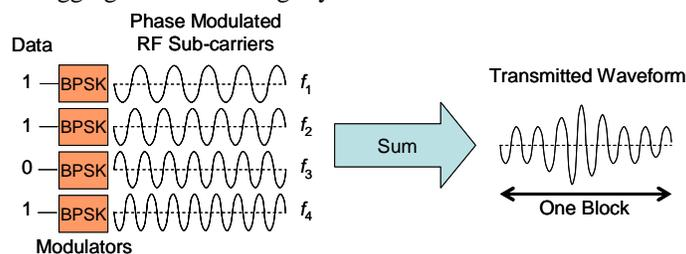
Fig. 1. Principle of OFDM transmitter illustrated with binary phase-shift keying.
