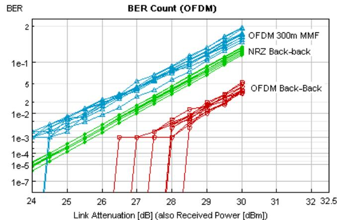
Fig. 7. BER versus link loss (1-mW transmitted power) for NRZ and OFDM systems.
