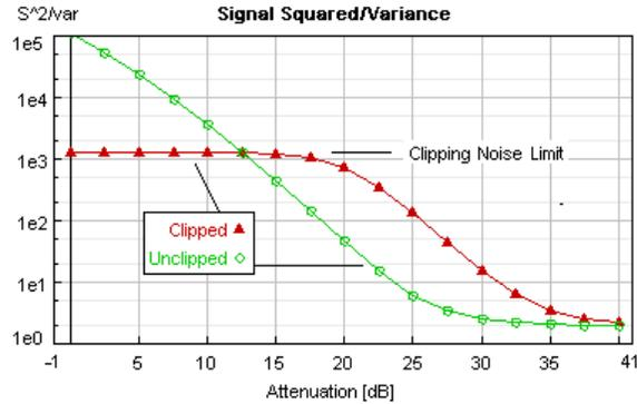
Fig. 5. Signal quality versus link attenuation for clipped and unclipped OFDM systems.
