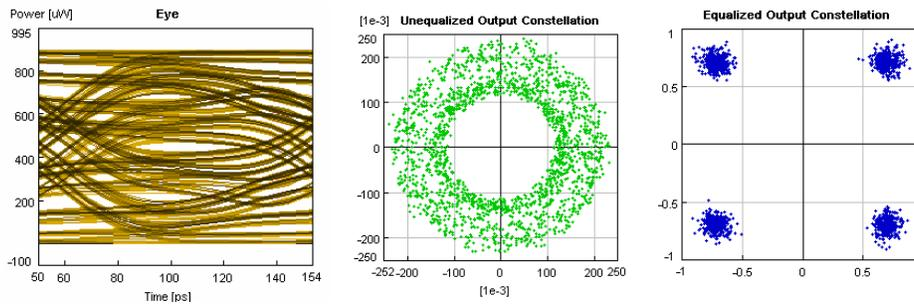
Fig. 6. (left) NRZ system; (centre) unequalized OFDM; (right) equalized OFDM.
