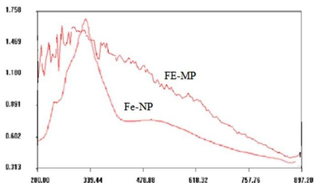
Fig. 1. UV Spectrum of synthesized iron oxide nanoparticles (Fe-NP) and iron oxide metalloprotein (Fe-MP)
