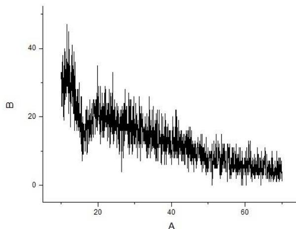
Fig. 3. XRD pattern of synthesized iron-oxide nanobiocomposite
