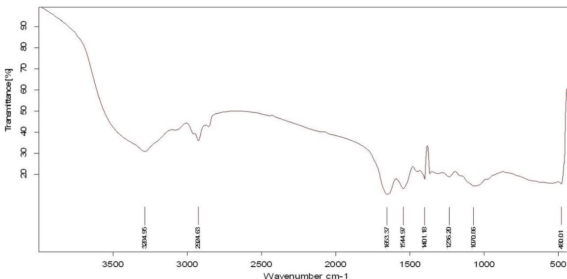
Fig. 2(b). FT-IR spectrum of synthesized iron-oxide nanobiocomposite
