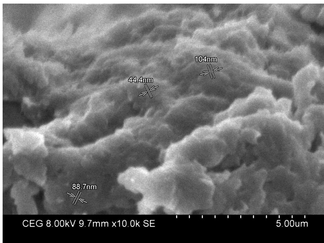
Fig. 4. SEM image of synthesized iron-oxide nanobiocomposite
