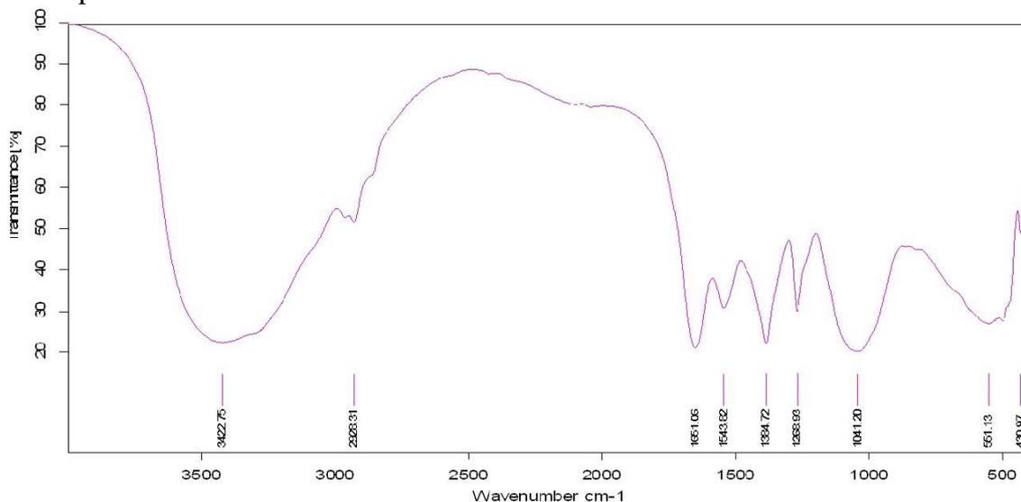
Fig. 2(a) FT-IR spectrum of synthesized iron oxide nanoparticles
