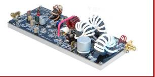
The RFP13.56-150XR is a high gain Class A/AB XR-rated amplifier designed specifically for the 13.56MHz ISM band. It is ideal as a driver stage or output PA in high power industrial, commercial, or scientific systems. Its XR rating ensures ruggedness when driving mismatched loads such as plasmas. It is supplied with SMA input and output connectors.
