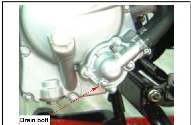
Refilling system with coolant and bleeding the air bubbles.
