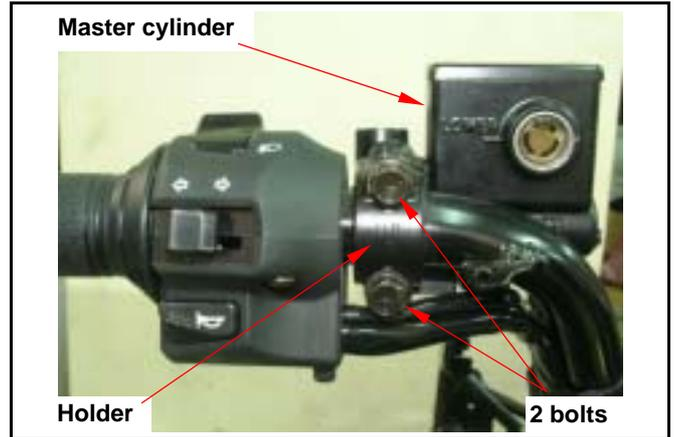
Loosen left handle switch connector.
