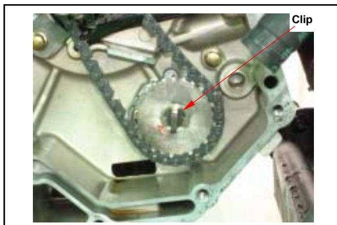
Make sure that pump shaft can be rotated freely. Remove 2 screws on the oil pump, and then remove oil pump.
