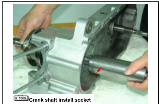
Turn in the crank shaft puller spiral tooth to the left crank shaft.
