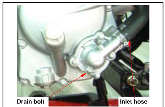
Remove the coolant inlet hose and thermo-sensor wire.
