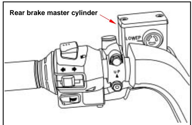
Remove the master cylinder cap and diaphragm. Increases the high quality brake fluid, uses by all means must with the trade mark brake fluid joins in the master cylinder. Clean the dirty brake disk.
