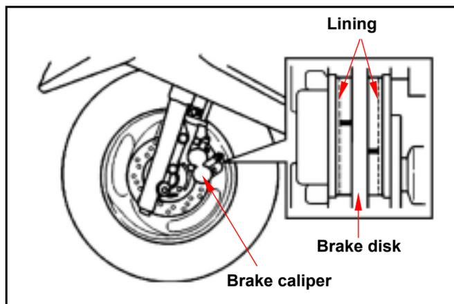
Remove the brake clipper bolt, and take out the clipper.
