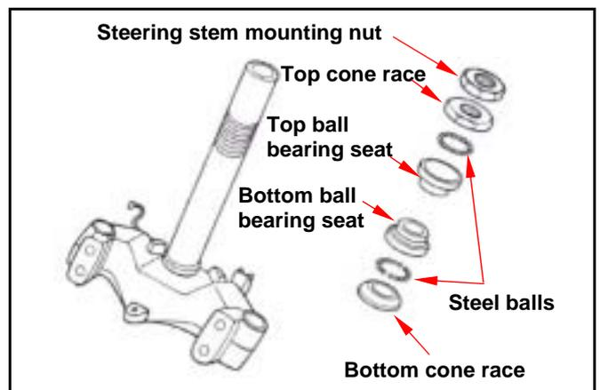
Lubricate the top cone race seat with grease. Screw the cone race in to top ball bearing seat till touching, and then screw out the cone race 1/4~3/8 turns.
