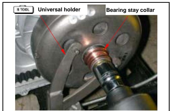
Install the drive face, washer and drive face nut. Hold drive face with universal holder, and then tighten nut to specified torque value.
