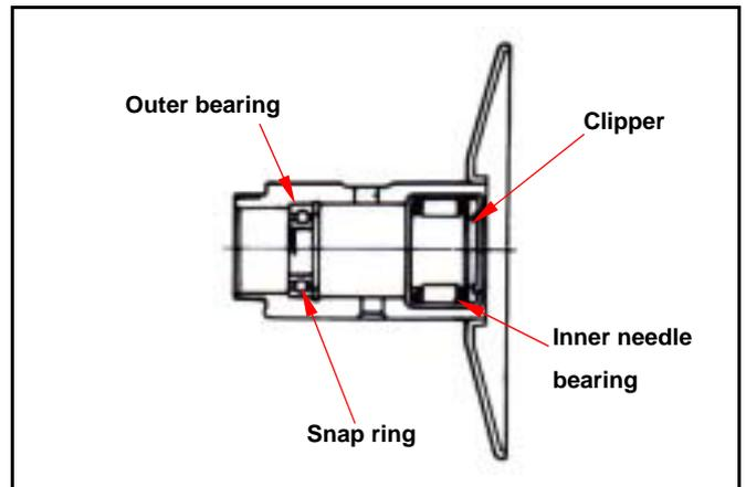
Remove snap ring and then push bearing forward to other side of inner bearing.
