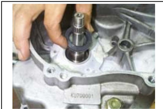
Install the oil seal in the left crankcase with special tool.
