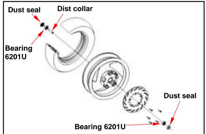
Install the brake disk and then tighten the bolts.
