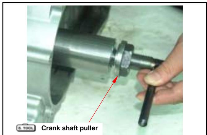
Hold left crank shaft puller, and turn the shaft puller nut by clutch nut wrench to pull in crank shaft into left crankcase.
