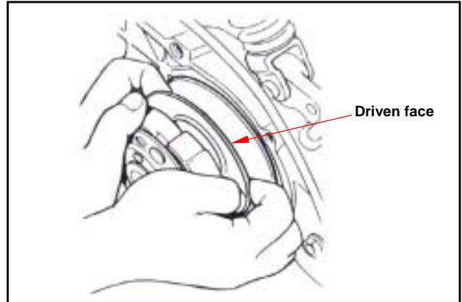
Install the driven pulley that has installed the belt onto drive shaft.
