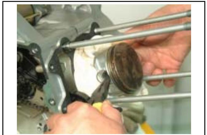
Remove cylinder gasket and dowel pin.
