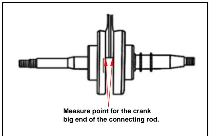
Measure the clearance of the big end at the vertical directions.
