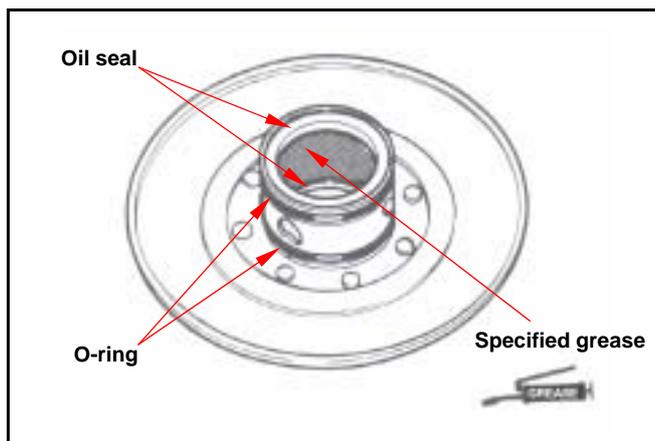
Install the movable driven face onto driven face.
