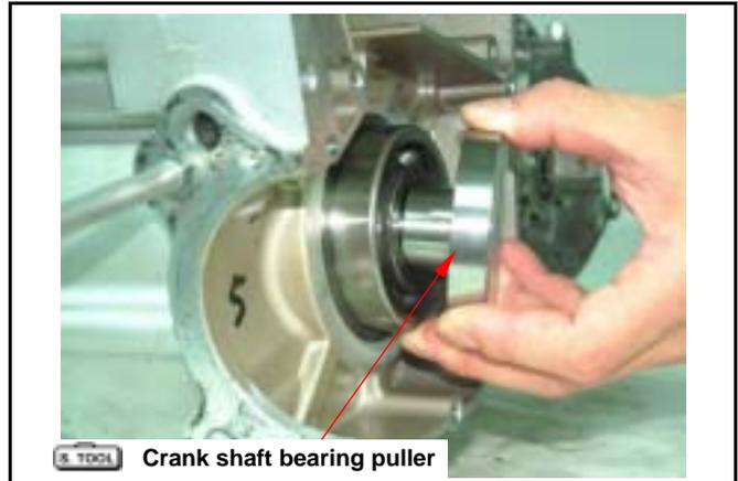
Install crank disassemble tool onto left crankcase. Install left crank shaft puller into crank case disassemble.
