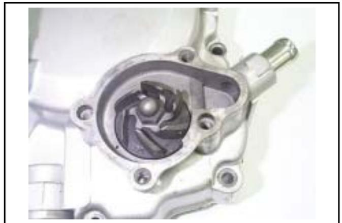
Install the dowel pin and new gasket.
