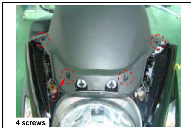
Loosen 8 screws from the inner box.
