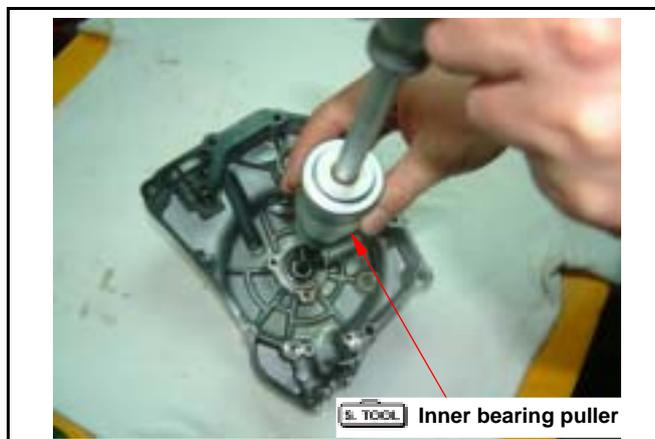
Install the bearing 6201 bearing with special tool.
