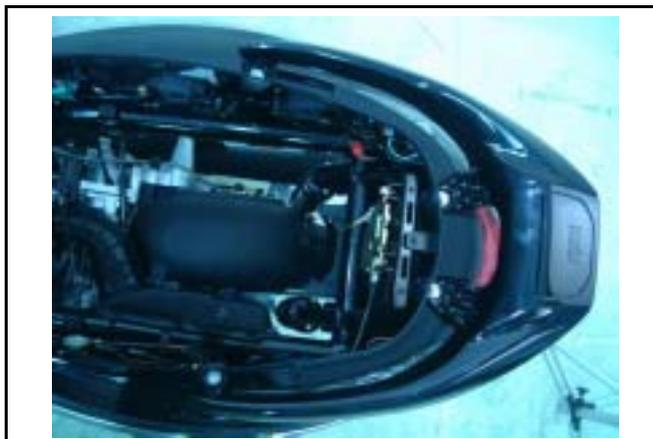
Remove right and left side covers (4 screws on each side.).
