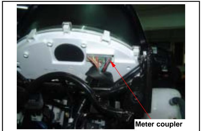
Loosen 4 screws from meter panel.
