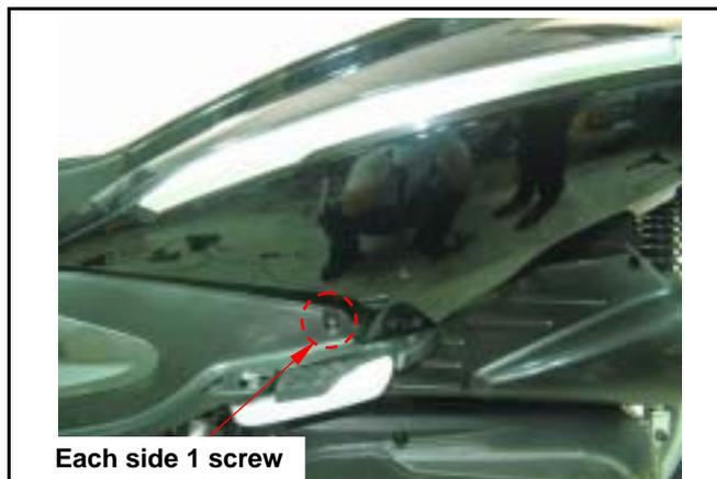
Loosen right and left side screws from rear side of the body cover.
