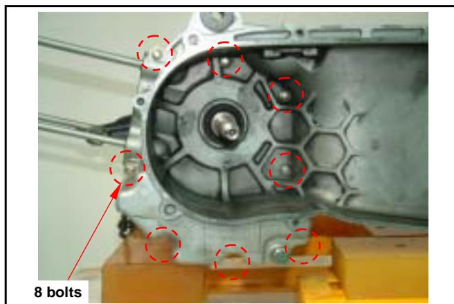
Place right crankcase downward and left crankcase upward.
