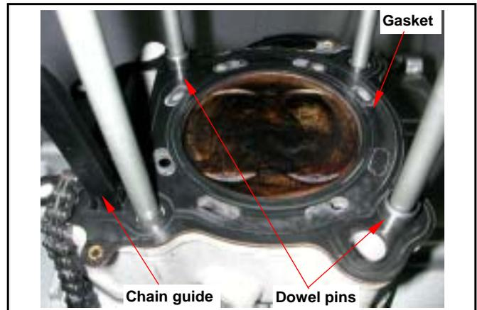
Install 4 washers and tighten 4 nuts on the cylinder head upper side, and then tighten 2 cylinder head mounting bolts of cylinder head right side.
