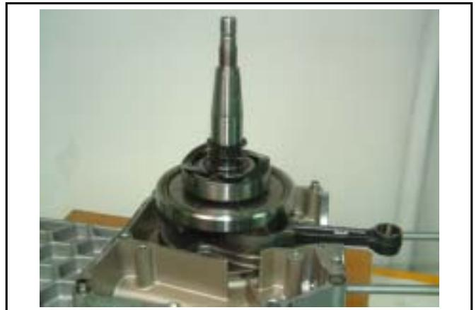
Install 2 dowel pins and new gasket.
