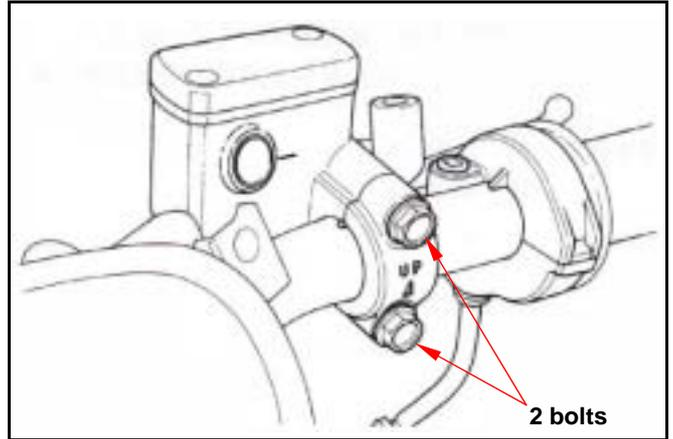
Connect brake hoses with 2 new washers. Tighten the brake hose bolt to the specified torque value. Make sure the hose is installed correctly. Install all wires, hoses, and components carefully so avoid to twisting them together.
