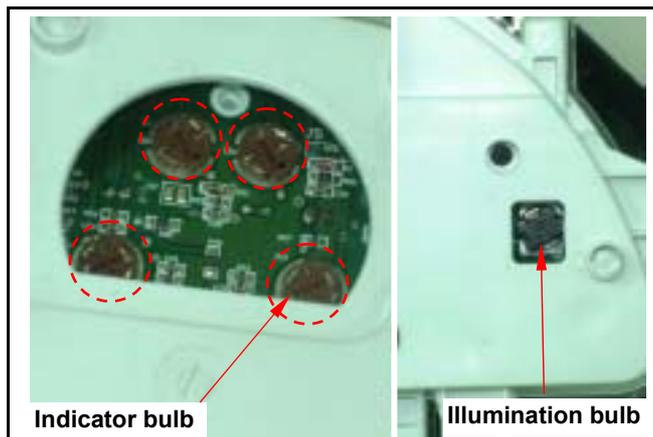
Uses the “-“ screw driver turn the indicator bulb seat in C.C.W. direction, and take out the indicator bulb.
