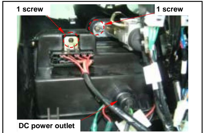
Loosen 1 screw from battery cover and remove it.
