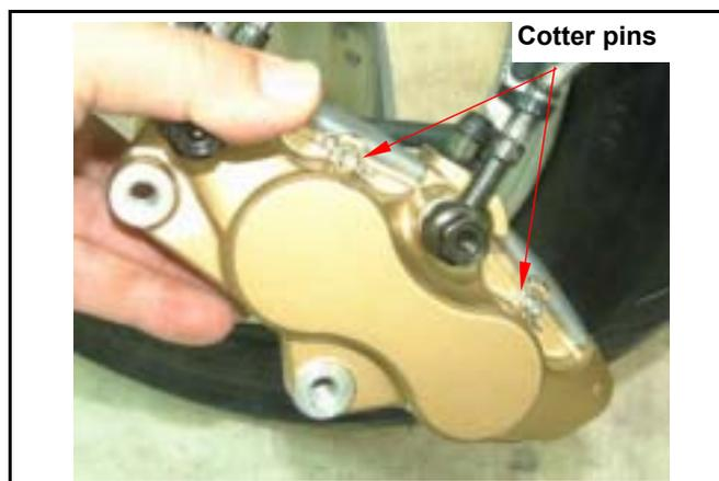
Remove the brake pad shafts and pads.
