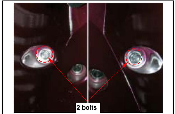
Loosen 2 screws and 2 bolts from the front cover upper side.
