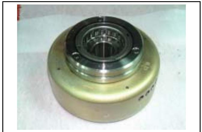
Install starting clutch driven gear onto one way clutch.
