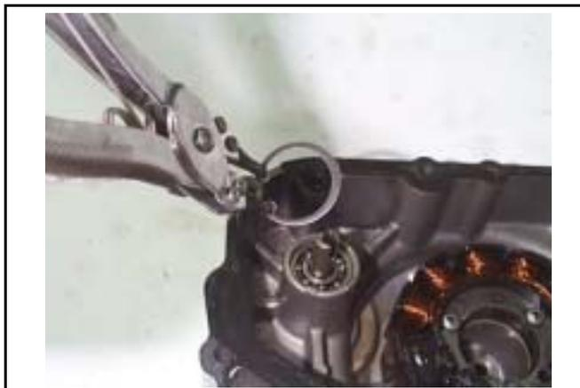
Install the seal washer into the rotor.
