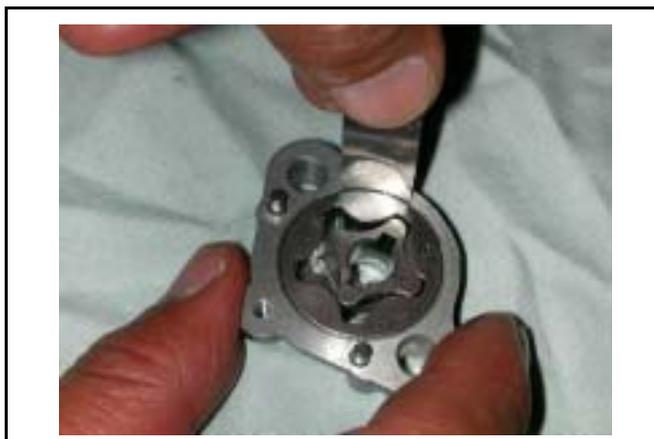
Check clearance between inner and outer rotors.
