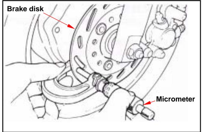
Remove the brake disk from wheel. Check the disk for deformation and bend.
