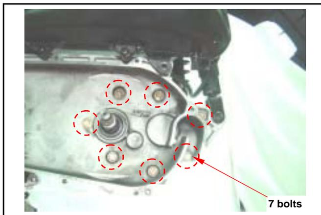
Remove the gear box cover.
