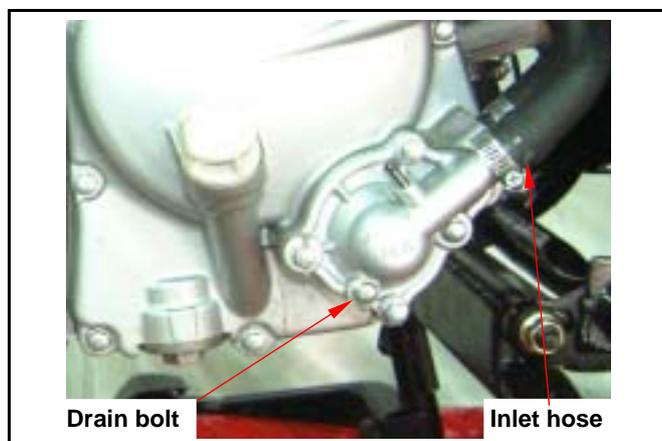
Remove the coolant inlet hose and thermo-sensor wire.
