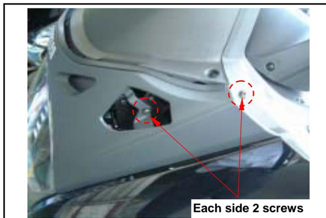
Loosen 8 screws from the wind screen and remove the wind screen.
