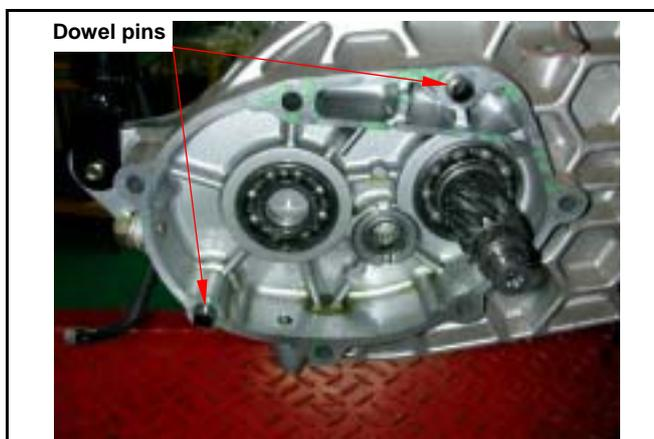
Install counter shaft and final shaft into the gear box cover.
