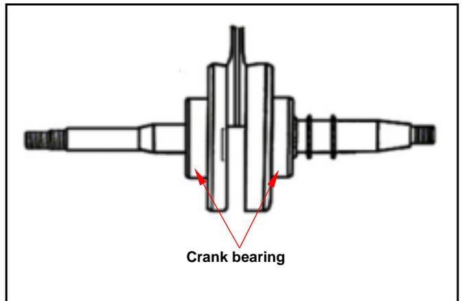
If any roughness, noise and loose linkage are detected, replace the bearing with new one.
