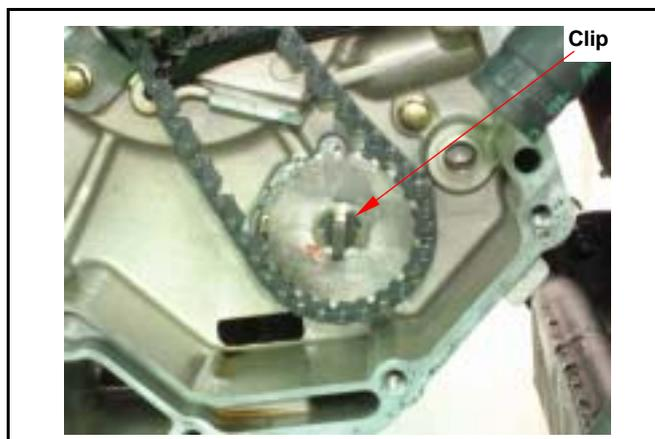
Install starting gear and generator.
