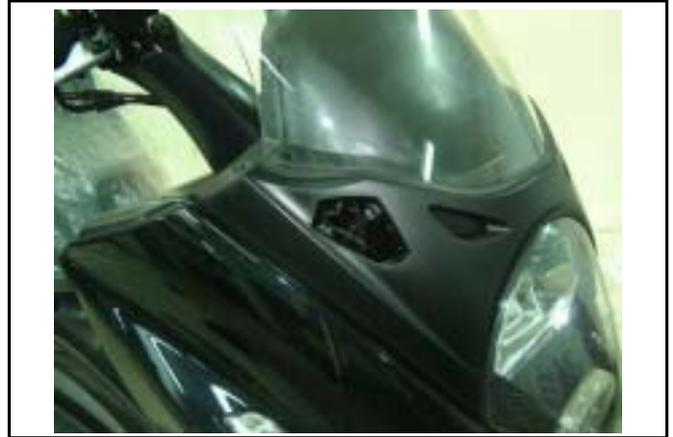
Disconnect the coupler of the speedometer, and take off the meter panel and meter.
