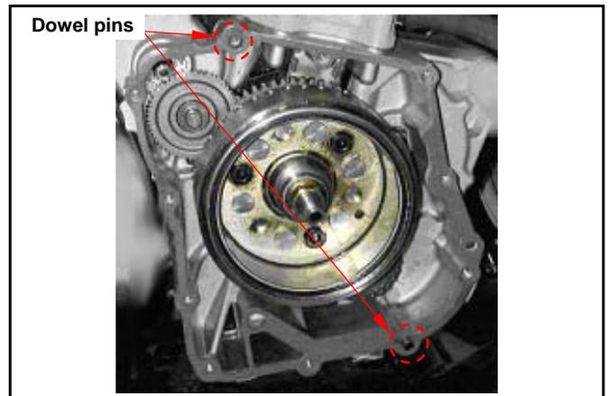
Install right crankcase cover (10 screws).
