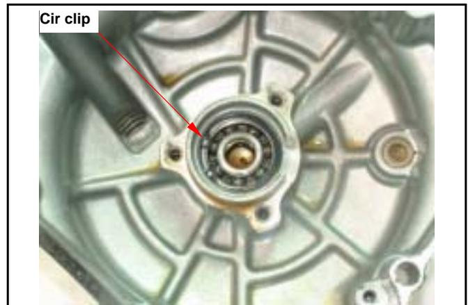
Remove the bearing 6201 with inner bearing puller.
