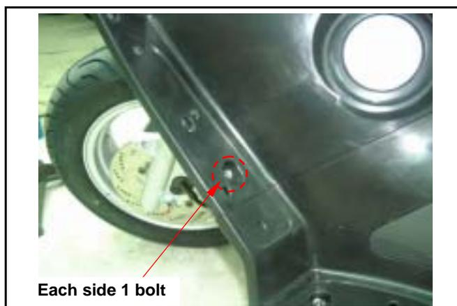
Loosen 2 bolts from inside of the inner box.
