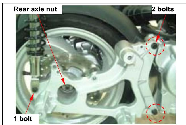
Remove the rear fork and rear axle collars.
