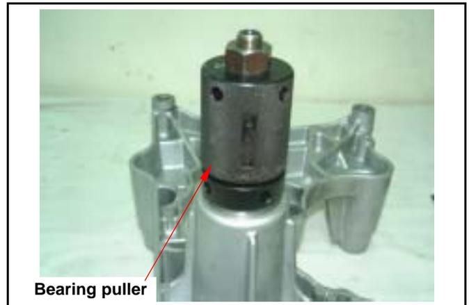
Use screw driver holder bearing puller lower part, and turn the bearing puller upper part to install the rear fork bearing.
