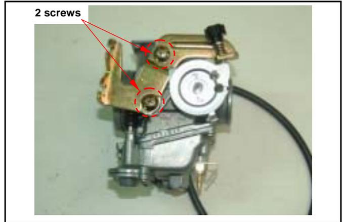
Remove the screws (2 screws) of the air cut-off valve and its cover.
