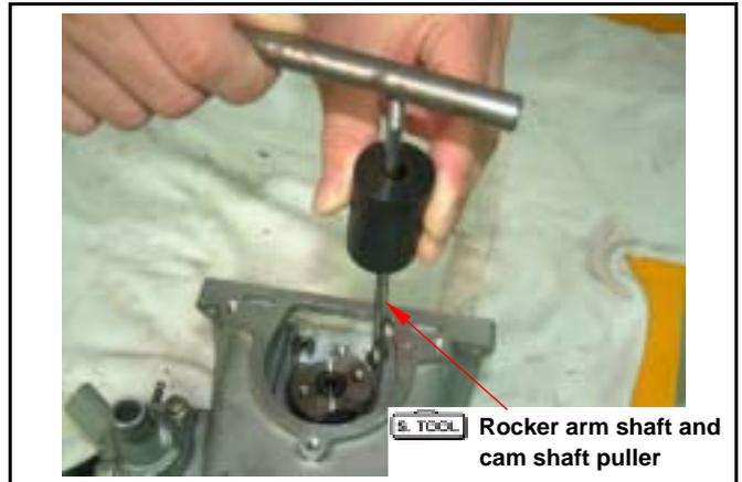
Remove cam shafts.
