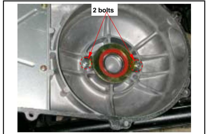
Check bearing on left crankcase cover. Rotate bearing's inner ring with fingers. Check if bearings can be turned in smooth and silent, and also check if bearing outer ring is mounted on cover tightly. If bearing rotation is uneven, noising, or loose bearing mounted, then replace it.
