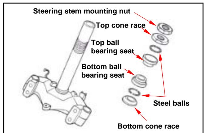
Lubricate the top cone race seat with grease. Screw the cone race in to top ball bearing seat till touching, and then screw out the cane race 1/4~3/8 turns.
