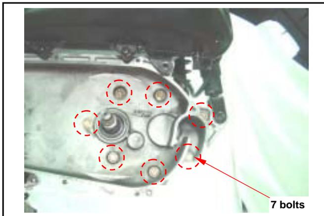
Remove the gear box cover.
