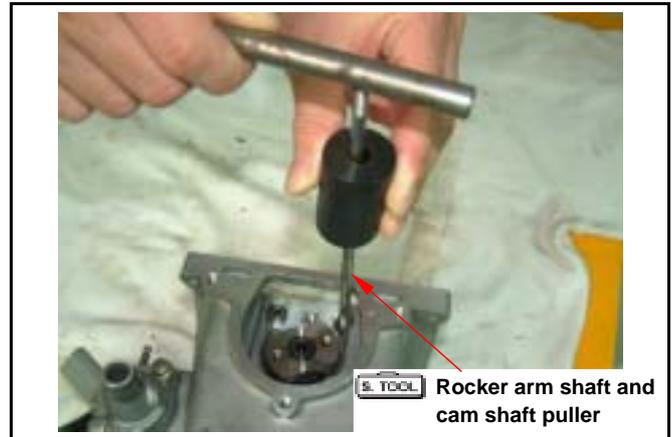
Remove cam shafts.
