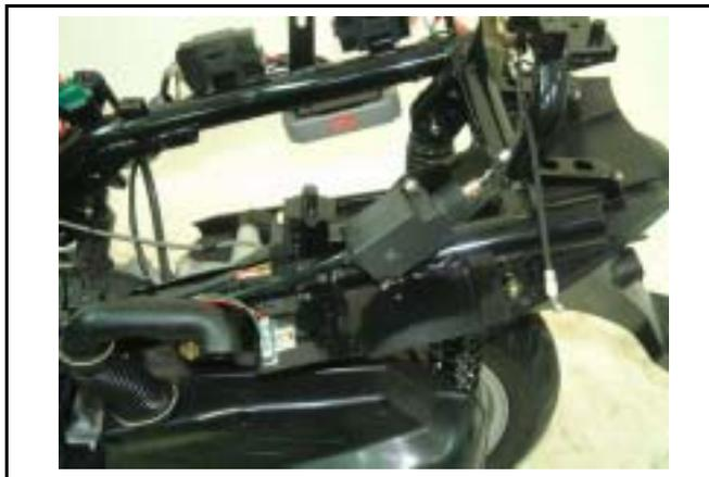
Remove the power coupler of auto by-starter.
