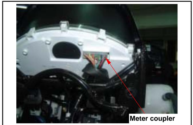
Loosen 4 screws from meter panel.
