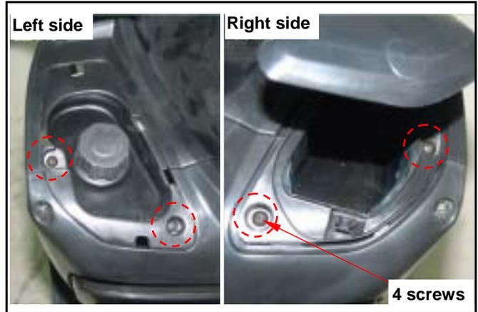
Loosen 2 screws from in side of meter panel.
