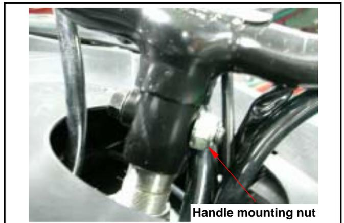
Apply with grease onto throttle cable and the sliding surface of handle.
