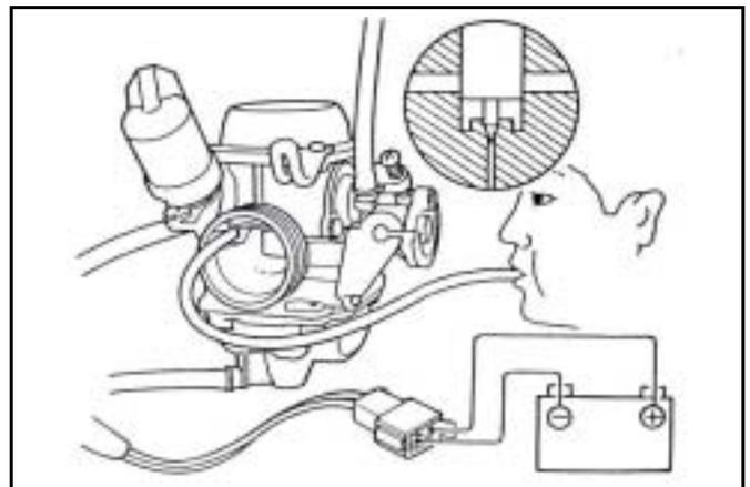
Connect battery posts (12V) to starter's connectors. After 5 minutes, test the rich circuit with compressed air.
