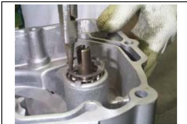
Check any wear and damage of the mechanical seal and inside seal.
