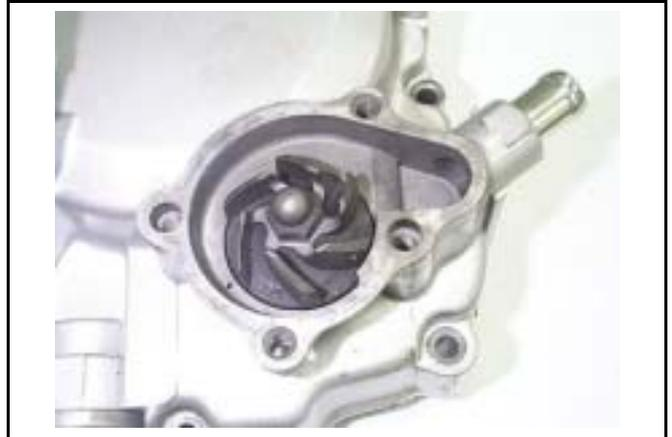
Install the dowel pin and new gasket.
