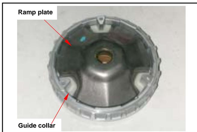
With 4~5g grease spreads wipes drives in the movable drive face axis hole.
