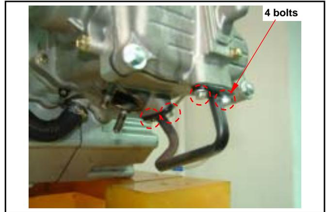
Remove the cylinder head side cover.
