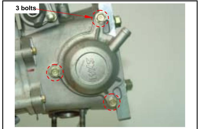
Remove left crankcase cover, and turn the Turn the drive face, and align the timing mark on the sprocket with that of cylinder head, piston is at TDC position.
