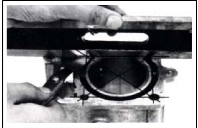
Measure clearance between piston rings and grooves.
