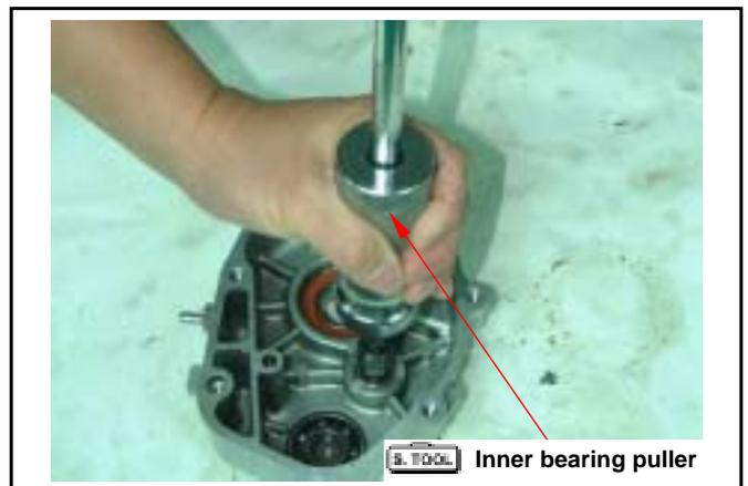
Remove oil seal, and then remove final shaft bearing from gear box cover using following tools.
