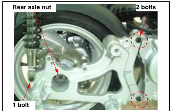
Remove the rear fork and rear axle collars.
