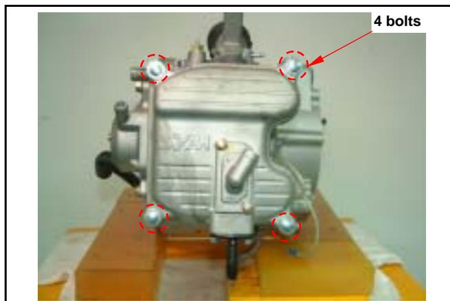
Install Air Injection system (AI) pipe. (4 bolts)
