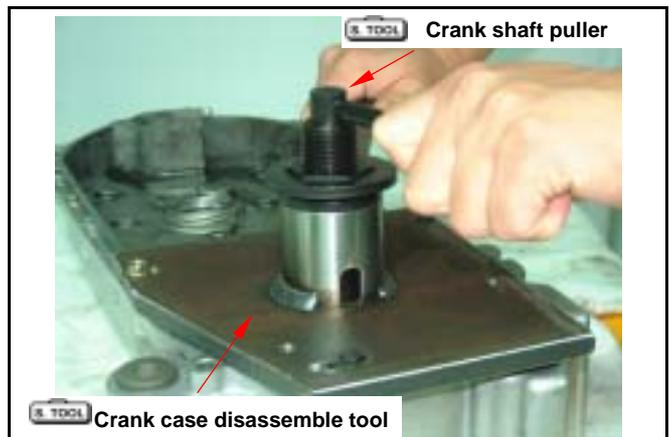
Install crank shaft onto the left crankcase and install crank shaft install socket.
