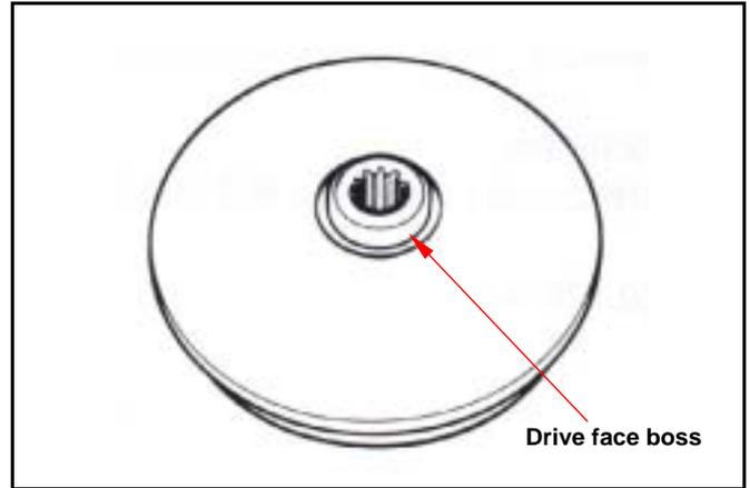
Install movable drive face comp. onto crankshaft.
