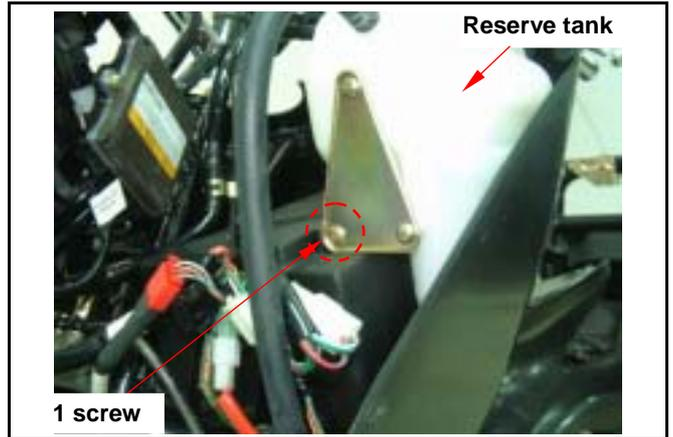
Loosen 1 screw from fuse box and remove it. Loosen 1 screw from main switch cap and remove the cap.
