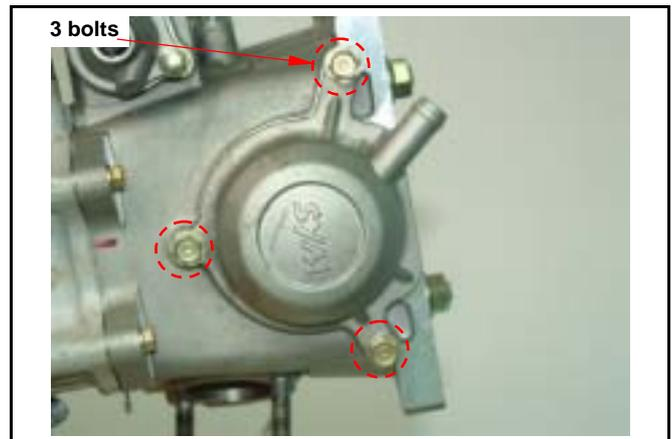
Remove left crankcase cover, and turn the drive face, and align the timing mark on the cam sprocket with that of cylinder head, piston is at TDC position.
