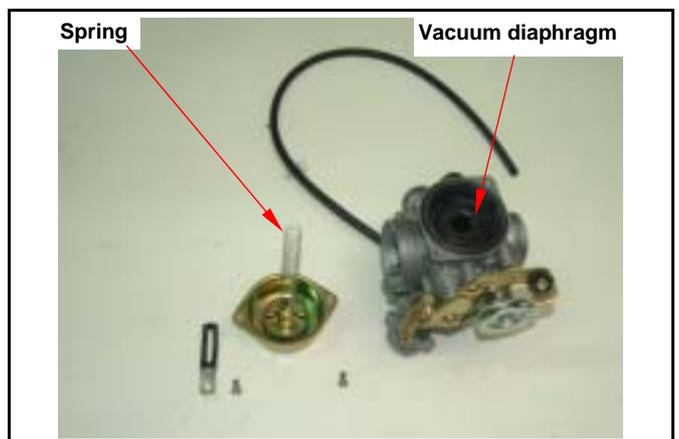
Remove fuel needle seat, spring, and injector needle.
