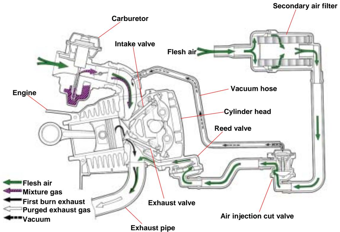
This system contained AICV (air Injection Cut Valve), R/V (Reed Valve) and other intake components.
