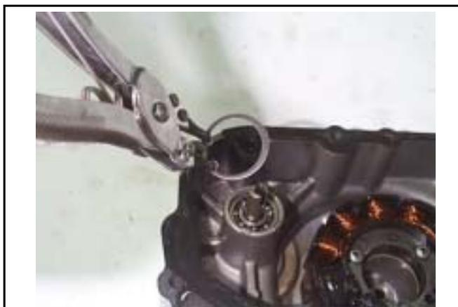
Install the seal washer into the rotor.
