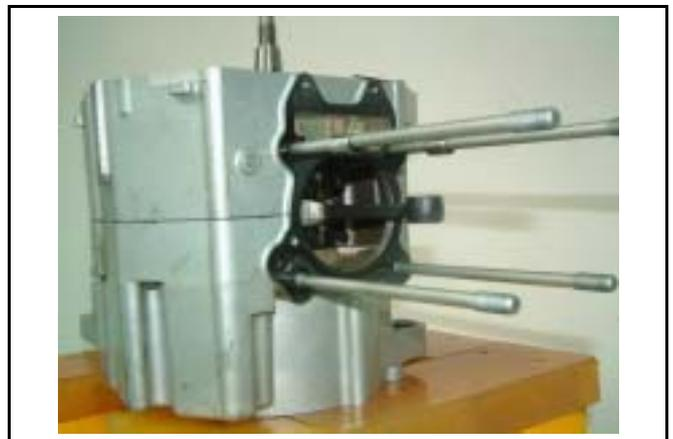
Tighten 8 bolts on the left crankcase.
