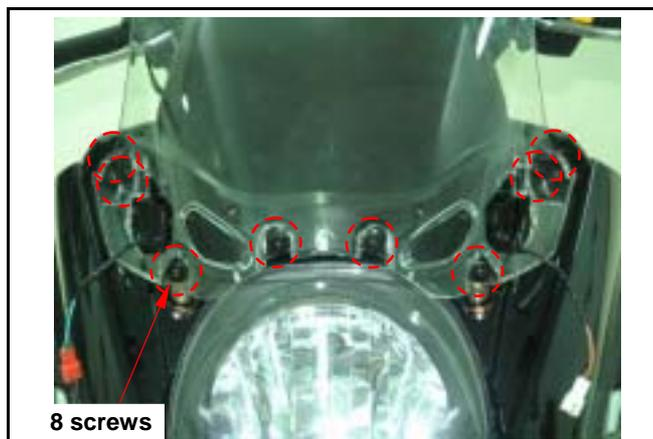
Loosen 4 screws from the meter visor and remove the meter visor.
