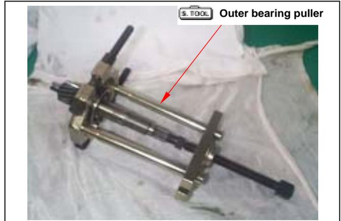
Remove final shaft bearing and counter shaft bearing from left crankcase using following tools.
