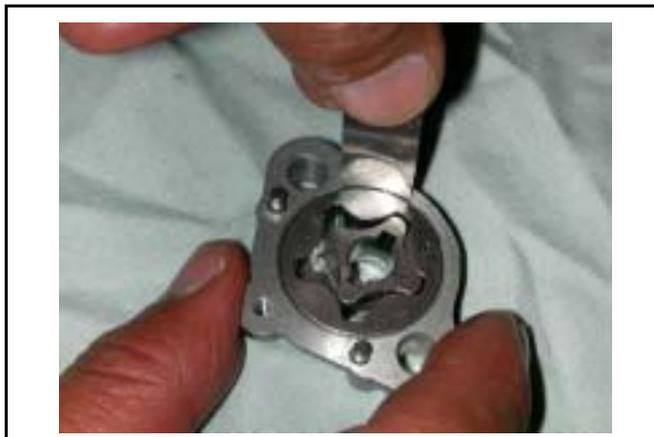
Check clearance between inner and outer rotors.
