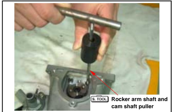
Remove cam shafts.
