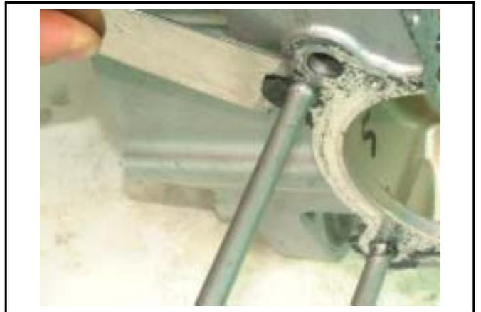
Install dowel pins and new cylinder gasket.
