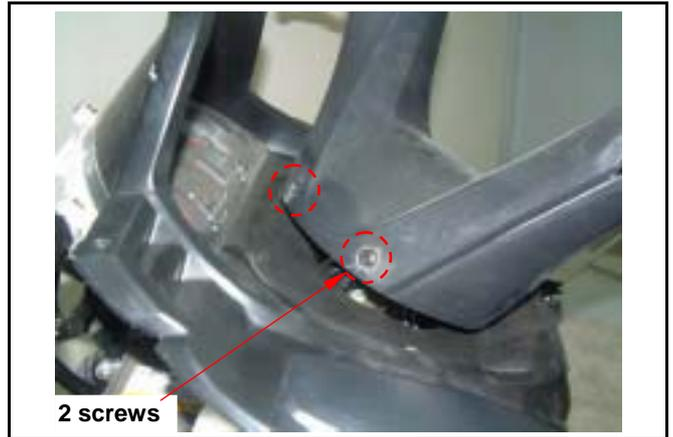
Loosen the 2 screws from handle upper cover rear end.
