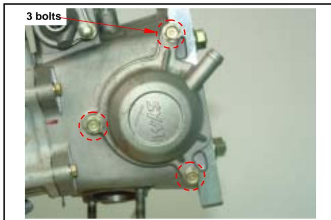
Remove left crankcase cover, and turn the crankshaft. Turn the drive face, and align the timing mark on the sprocket with that of cylinder head, piston is at TDC position.
