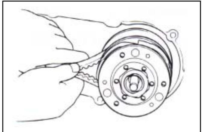
Install the clutch outer and bearing stay collar. Hold the clutch outer whit universal holder, and then tighten nut to specified torque value.
