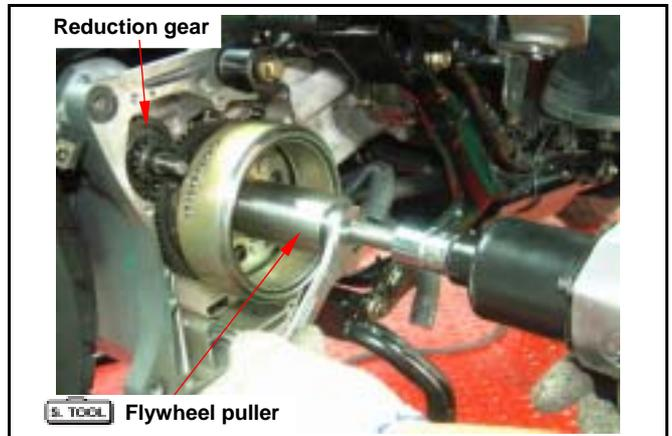
Remove flywheel and starting driven gear.
