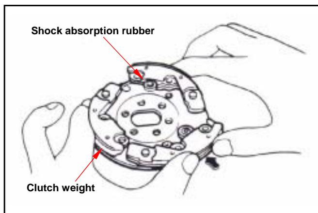
Install the spring into groove with pliers.
