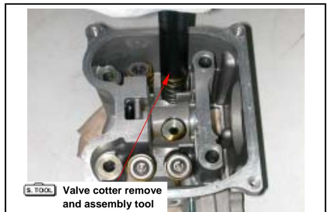
Remove valve cotters, spring retainers, springs and valves.
