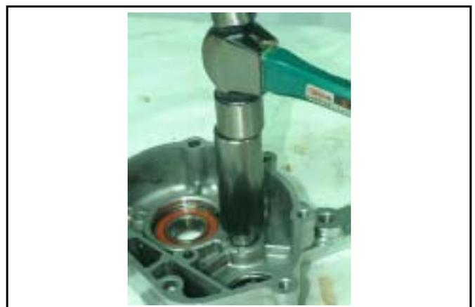
Install new final shaft bearing and bearing puller onto left crankcase.
