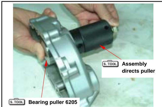
Use screw driver holder bearing puller lower part, and turn the bearing puller upper part to install the final shaft bearing.
