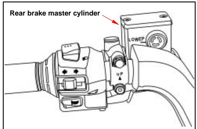
Remove the master cylinder cap and diaphragm. Increases the high quality brake fluid, uses by all means must with the trade mark brake fluid joins in the master cylinder. Clean the dirty brake disk.
