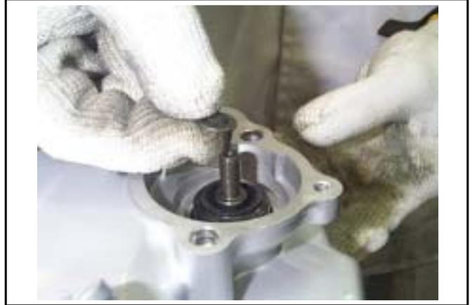
Install the rotor onto the water pump shaft and tighten.
