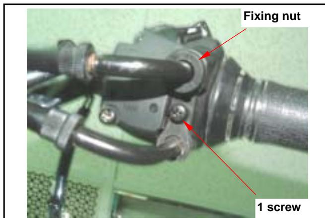
Loosen 2 screws from the throttle holder.
