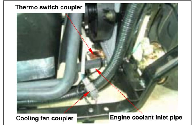
Remove reserve tank coolant inlet pipe.
