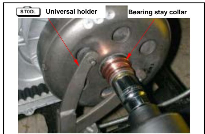
Install the drive face, washer and drive face nut. Hold drive face with universal holder, and then tighten nut to specified torque value.
