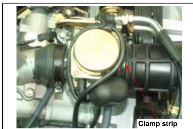
Remove the air cleaner inlet pipe connection bolt (1 bolt).
