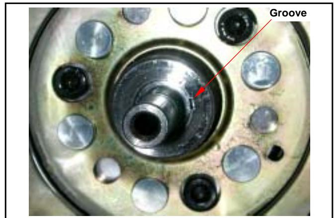
Hold the flywheel by drive face with universal holder, and tighten flywheel nut.
