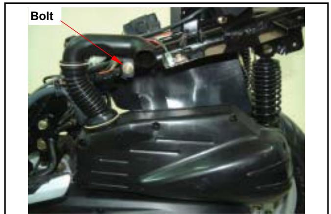
Remove 6 screws, and then remove the air cleaner element.
