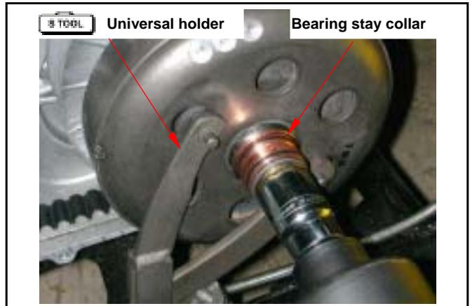
Push the drive belt into belt groove as diagram shown so that the belt can be loosened, and then remove the driven pulley.
