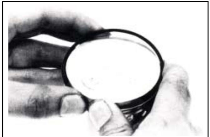
Place piston rings respective into cylinder below 20 mm of cylinder top. In order to keep the piston rings in horizontal level in cylinder, push the rings with piston.
