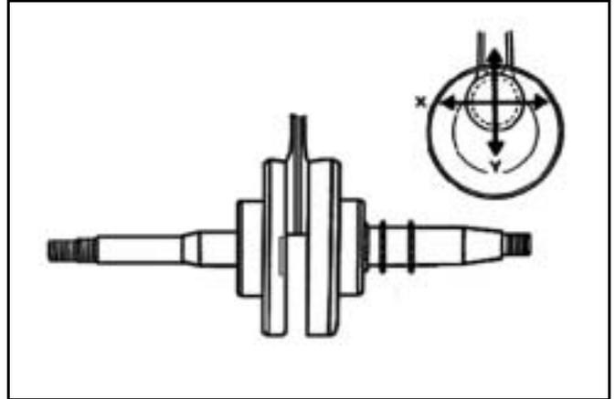
Place the crankshaft on a V-block, measure run-out of the crankshaft.
