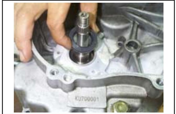
Install the oil seal in the left crankcase with special tool.
