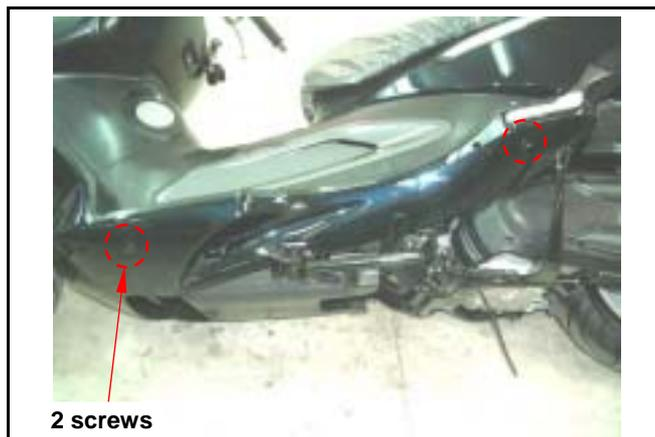
Loosen 2 screws from the side cover upper end.
