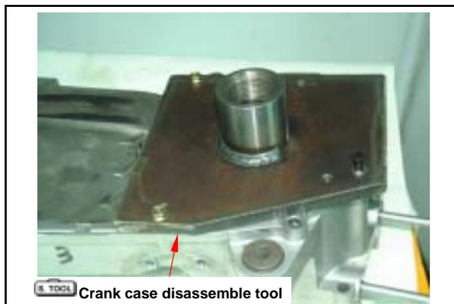
Install left crank shaft puller into crank case disassemble.
