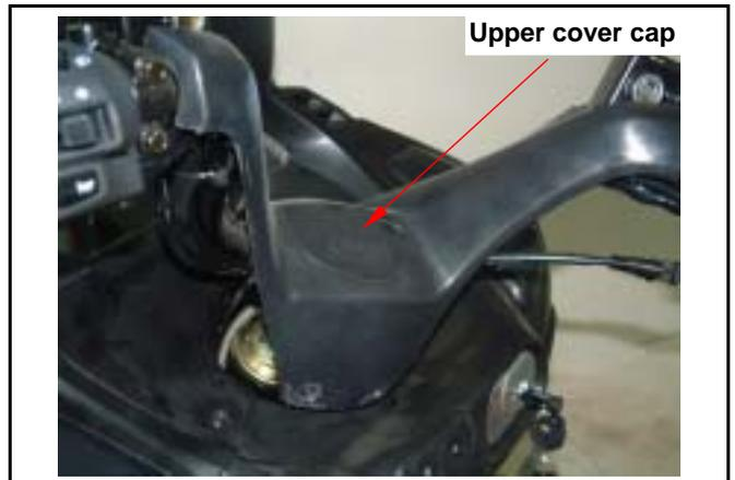
Loosen the 3 screws from the handle upper cover, and then remove handle upper cover.
