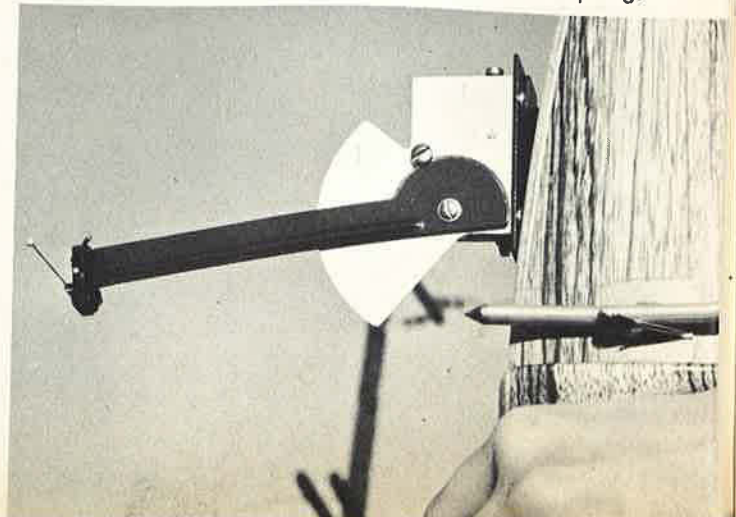
As shown, fletching on arrow will simply brush the bead of the sight out of its way, bending the spring.
