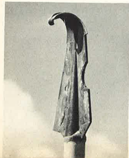
Below: A miss on a sage hen can have bad effect on a broadhead. This one was bent in ricochet against a rock.
