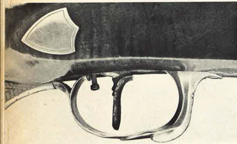
This miniature crossbow features a set trigger, which can be adjusted to trip the mechanism at light touch.
