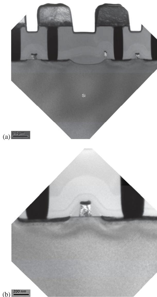
Figure 5: (a) Low magnification TEM image of the EXpressLO™ specimen manipulated and FIB milled in a backside orientation shows the elimination of curtaining artifacts. (b) TEM image of the gate region in the backside prepared specimen.
