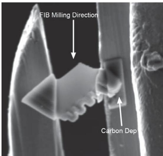
Figure 4: Optional ion beam assisted carbon deposition further secures the specimen to the grid. Then the backside oriented specimen is FIB milled to electron transparency from the Si side of the specimen.
