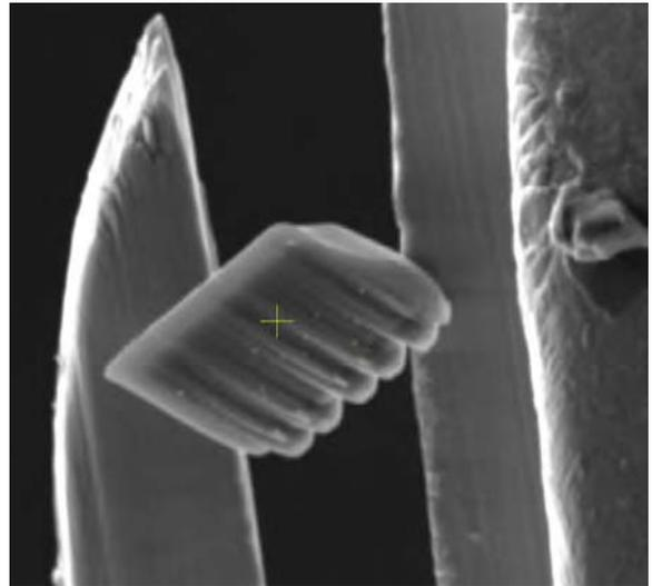
Figure 3: An SEM image of an EXpressLO<sup>TM</sup> specimen manipulated into a backside orientation after the grid/specimen assembly is put back into the FIB/SEM for further thinning.
