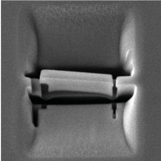
Figure 1: An example FIB milled specimen ready for EXLO. The specimen is 1-2  $\mu\text{m}$  thick.
