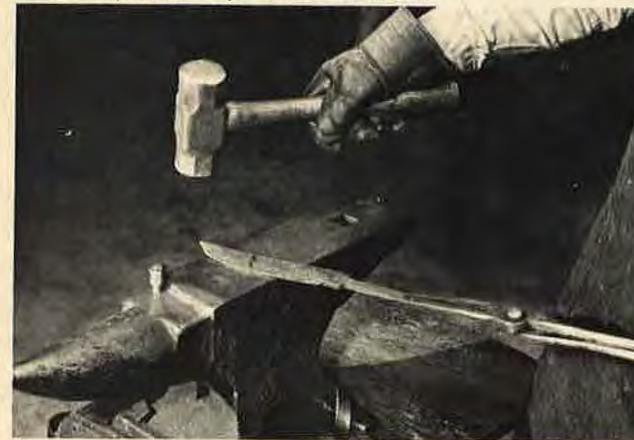
Actor Robert Middleton, currently in ABC's "Monroes" TV series, uses this knife for many purposes. (Below) In forging, Swedish tool steel is used to form the rough blade. It later is hardened, then tempered in oil bath.
