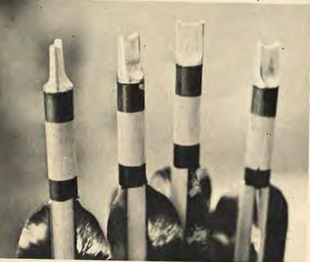
Above: The bolts at top are efficient, but Army personnel felt that the shaft at bottom was more in keeping with the needs of a combat arm. (Left) Nocks on the bolts developed for experimentation are of tough alloy material.
