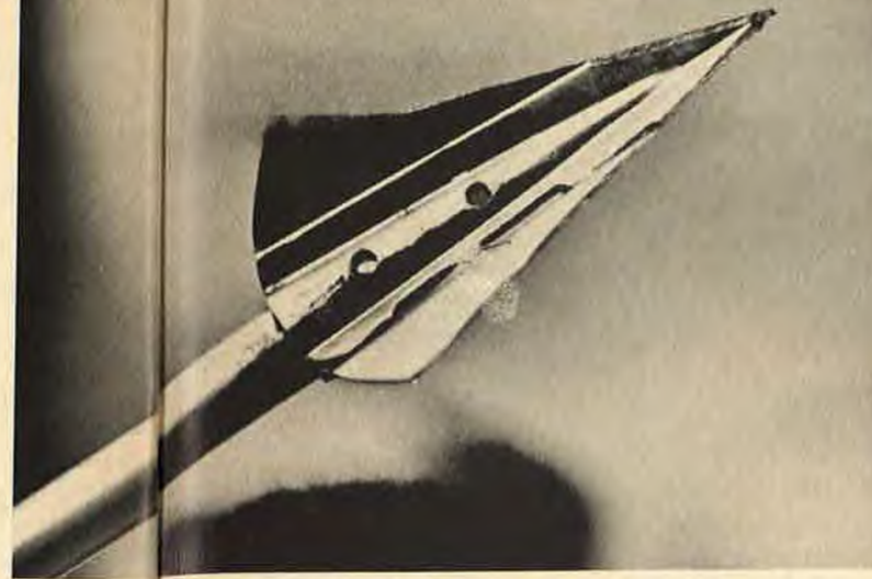
Above: The bolts developed for experimental combat use in the Vietnamese jungles were tri-bladed broadheads of familiar design. (Right) On the latest 150-pound crossbow developed for Vietnamese use, Benedict has installed this heavy-duty bowsight.
