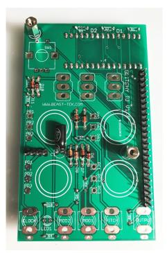
**IMPORTANT** – Do NOT solder any of the switches, pots or rotary encoder in place until the front panel is on!!! Soldering them on now will make assembling the front panel extremely difficult.
