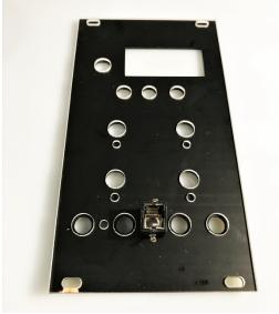
Once all five jacks are installed, make sure that the pins are all straight and make sure the jack bodies are aligned nicely. Bend the ground connector on each of the jacks at approximately 45 degrees as per the photos.
