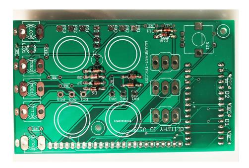
Install the 220 ohm resistors R1, R2, R3 and R4 on to the BACK of the PCB (no silk screen side). Install the 10K resistor R11 on to the BACK of the PCB (no silk screen side). Solder in place, trim leads.
