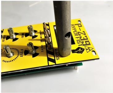
Place washers and nuts onto the 4 pots. Tighten the nuts, again using a tube spanner or ring spanner to avoid scratching the front panel.
