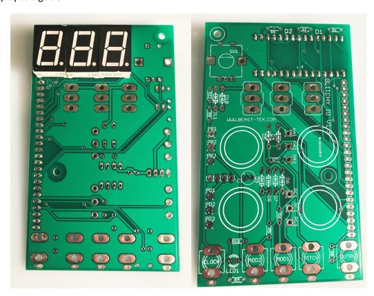
Once the orientation has been confirmed, solder one lead from each display and check that they sit flush with the board. If they are not flush, they can be adjusted easily by heating the single solder joint and maneuvering them into place. Once you are happy, solder the rest of the leads and trim.
