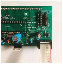
Once the IDC socket orientation has been confirmed using the power cable, solder the remaining pins.
