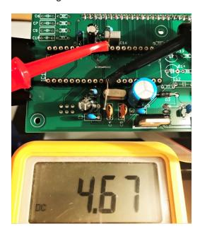
If these voltages do not check out, double check all solder joints and check the orientation of the voltage regulator (IC3) and the power diodes.
