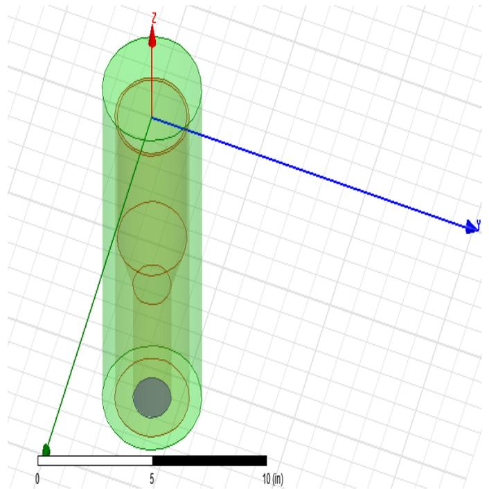
Fig.1: Geometry of Conical horn antenna
