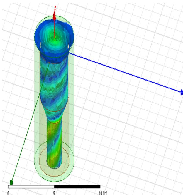
Fig.5: Radiation Pattern of Conical Horn Antenna
