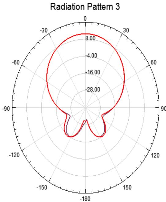
Fig.2: Directivity of a Conical horn antenna of RHCP
