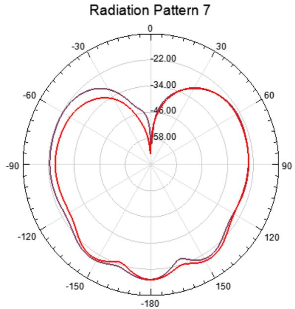
Fig.3: Directivity of a Conical horn antenna of LHCP
