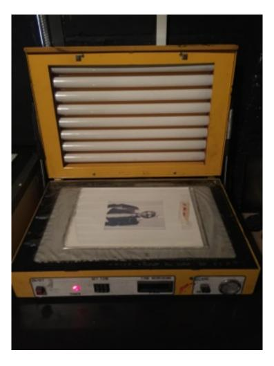
Once dry the negative can be placed on the paper and a contact print made by inspection in sunlight or under an ultra-violet lamp, until the image is 1/2 stop over-exposed..
