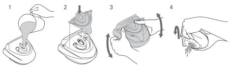
Wash the water chamber, spill guard, tub plate and tub plate seal in warm water, using a mild detergent. Use the yellow cleaning plug to assist in the cleaning process (see steps 1 to 4). Rinse thoroughly in clean water and allow them to dry away from direct sunlight.
