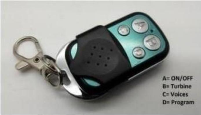
Press "A" 1 time = on/off scanner (if REM is disconnected)
