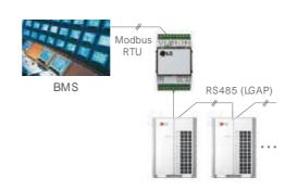
Max. 64 indoor units with 4 modules in one Modbus communication line
