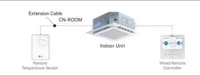
This installs easily and discreetly into a wall and then connects to indoor unit
