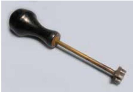
If you'd like to try one, all you need is a little scrap copper or nickel about 22-24 gauge, a piece of heavy brass or copper for a base, about 6 inches of metal rod and a piece of wood for the handle.
