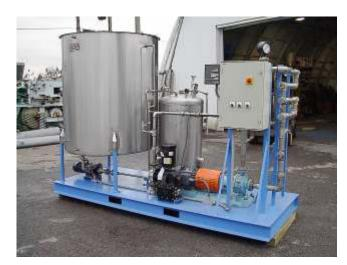
**Biodiesel Skid** - Fabricated for a biodiesel system OEM. Features new control panel, refurbished tank, and special mixing system.
