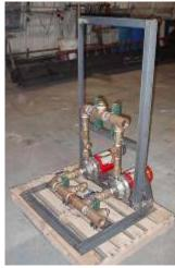
**Two Small Pump Skids** - Stainless steel frames, stainless and copper piping with valves from TriStar
