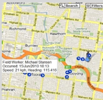
The 'Breadcrumb' trail view shows speed, direction, location, and status of workers
