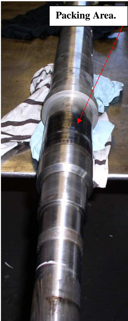
Figure 21. Shaft Packing Area Discolored by Packing Rubbing.
