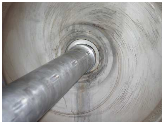
Figure 44. Shaft Keyways Machined in Alternating Arrangement. Keys Transfer Torque to the Impeller Hubs.
