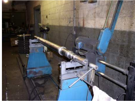
Figure 46. Bare Shaft in Balancing Machine. Impellers Are Stacked at the End of the Balance Machine.
