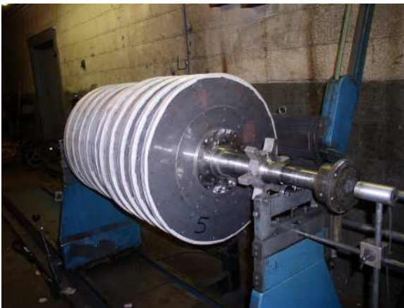
Figure 47. Rotor Stacked, Impellers Taped For Wind Resistance For Balancing.
