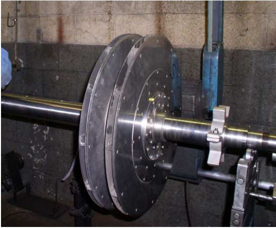
Figure 45. Impellers Being Installed on Shaft.
