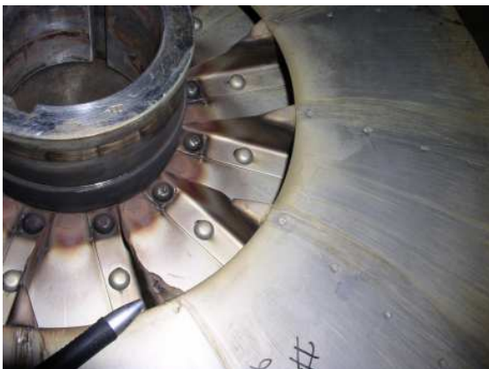
Figure 43. Impeller #2 Blade Damage. Note Heating of the Hub Which Occurred During Previous Assembly.
