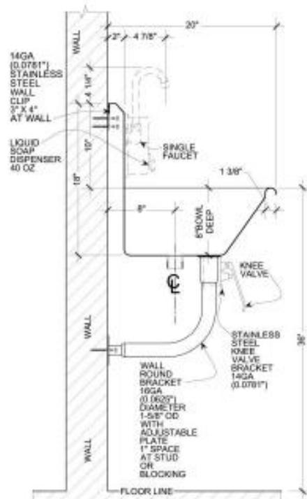
**Engineering Specification:** 14 gauge, type 304 stainless steel wash sink. 1-3/8" rolled rim. 1-1/2" welded in drain. Exposed surfaces polished to a satin finish. Supported on (2) wall clips. Legs to wall.
