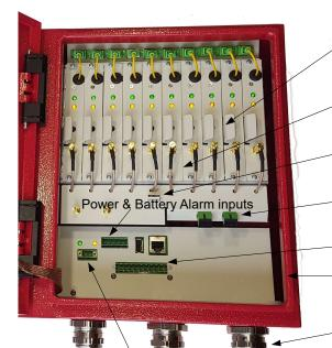
Opto-Channelized <sup>TM</sup> cards 1 frequency per card, ´any band, individual channel control
