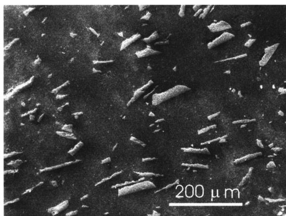
FIG. 1. SEM image of sample 2401 showing inhomogeneous distribution of MQP-Q ribbons.
