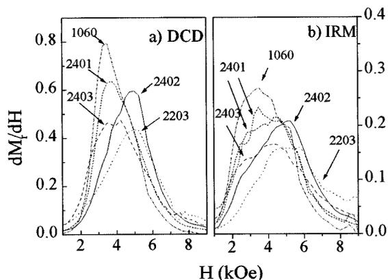
FIG. 3. IRM and DCD susceptibilities of the bonded magnets studied. For magnet 2401, the two IRM curves are for different samples and show different structure.
