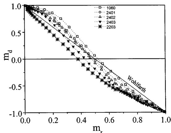
FIG. 4. Henkel plots for all samples, in which the reduced DCD remanence is given as a function of the reduced IRM remanence.
