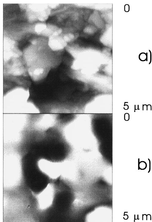
FIG. 2. (a) AFM image of the  $5\ \mu\text{m} \times 5\ \mu\text{m}$  region of Ba ferrite in sample 2401. (b) MFM image of the same  $5\ \mu\text{m} \times 5\ \mu\text{m}$  region showing stray magnetic fields present in the sample. Note that the magnetic domain structure does not coincide with the grain structure.
