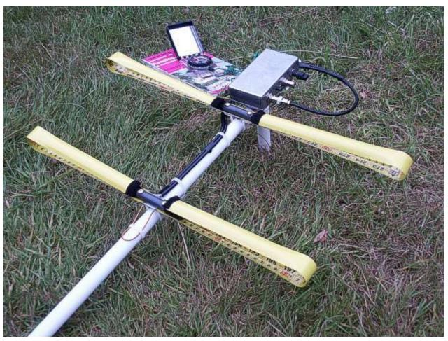
Attenuators are used when approaching the near vicinity of a transmitter to keep the received signal strength within a usable S-meter range.
