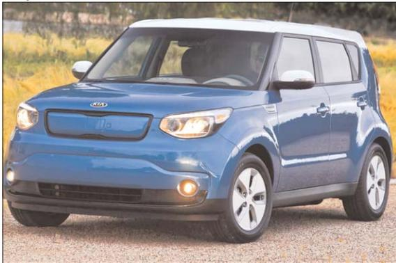
Kia Motors has brought out an electric version of its Soul crossover. The Soul EV features two standard charging ports, an SAE J1772 port for Level 1 and Level 2 AC charging, and a CHAdeMo DC fast-charging port (480 V). It can be charged to 80 percent in as little as 33 minutes with a 50 KW fast charger
