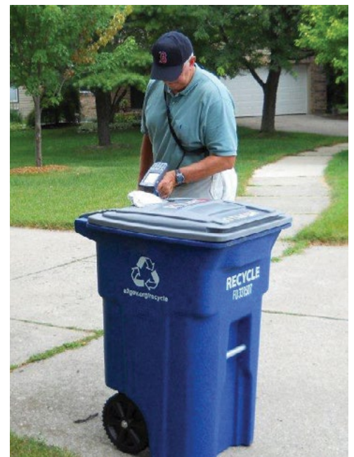
Toter's RFID solution includes handheld RFID/barcode scanners for delivery data collection, cart maintenance, and inventory control.
